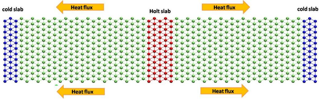
**Figure 2:** Schematics of the reverse non-equilibrium MD simulation
