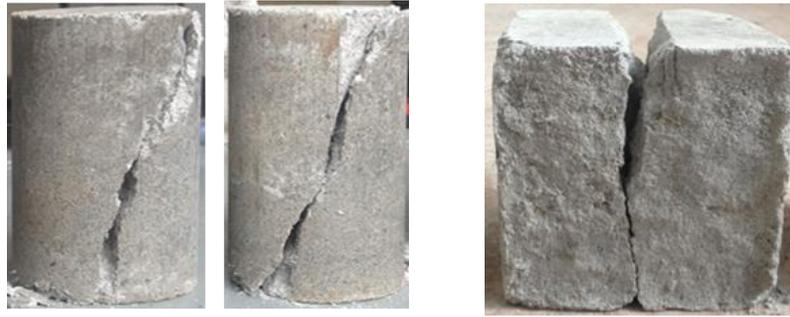
(a) Uniaxial compression testing samples (b) Brazilian split testing samples
