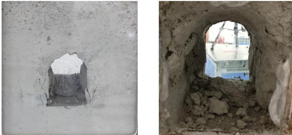
(d)  $\sigma_z=1.333$  MPa
