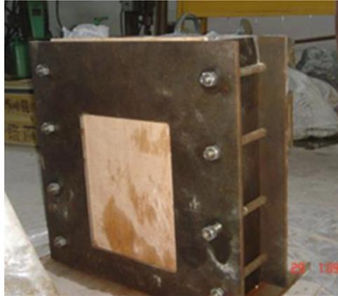
**Figure 3:** Fixed steel plates and the testing boundary conditions
