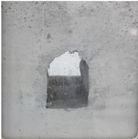
(c)  $\sigma_z=1.167$  MPa, excavation completed.
