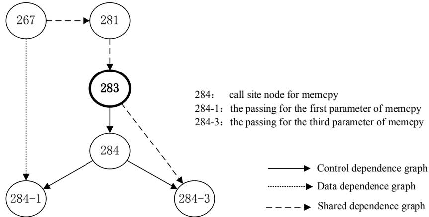
**Figure 4:** Enhanced system dependency graph for code snippet 1
