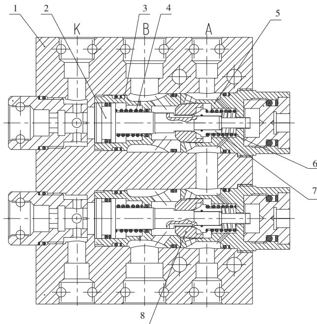
**Figure 1:** Schematic diagram of water-medium high-flow hydraulic one-way valve. 1. Valve body, 2. Piston, 3. Valve seat, 4. Return spring, 5. Valve sleeve, 6. Valve core return spring, 7. Pilot valve core and 8. Main valve core
