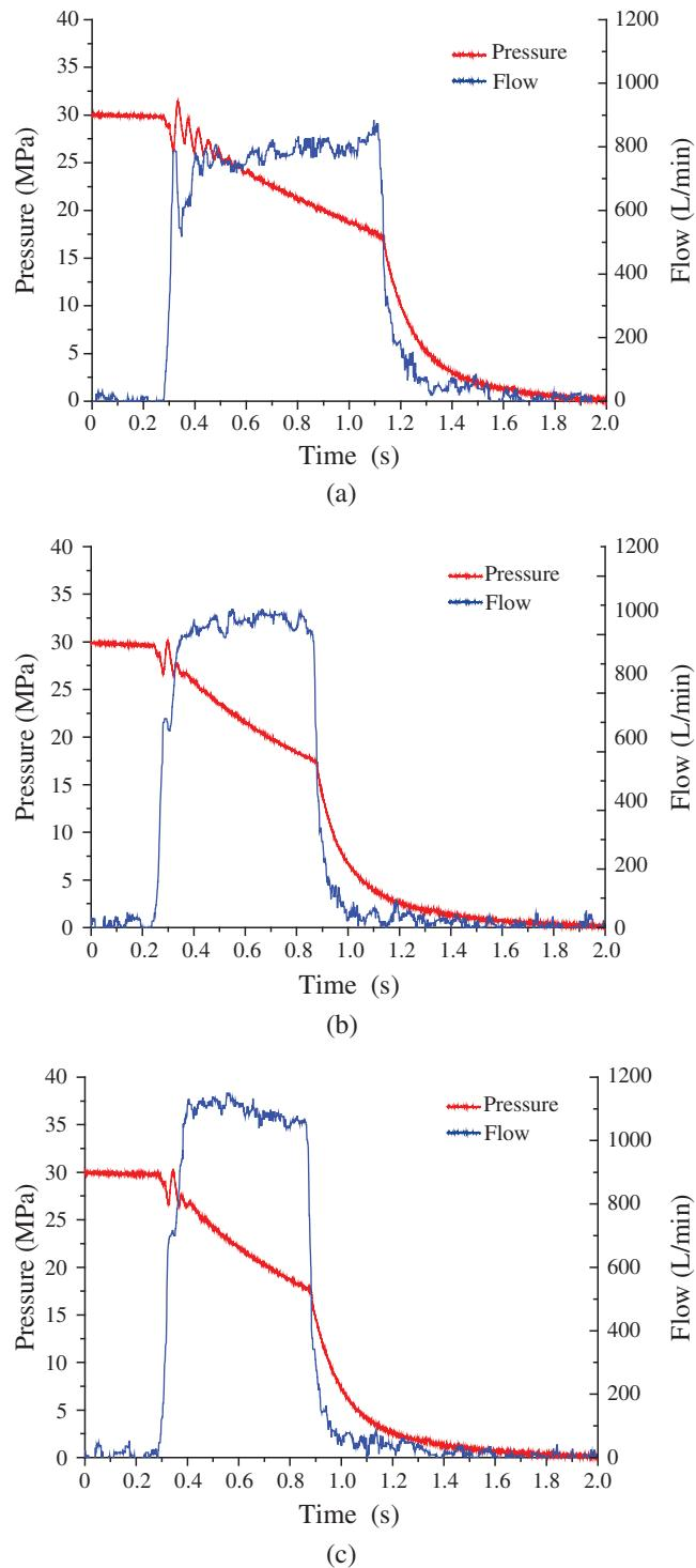
**Figure 8:** Impact characteristics for different control pressures. (a) 12 MPa, (b) 14 MPa and (c) 16 MPa
