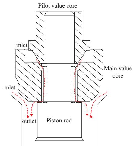
**Figure 3:** Main valve core opened
