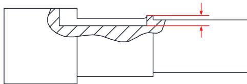
**Figure 6:** Through-flow keyway on the valve stem
