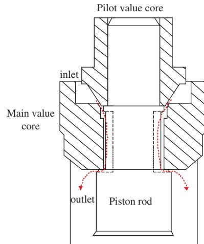
**Figure 2:** Pilot valve core opened
