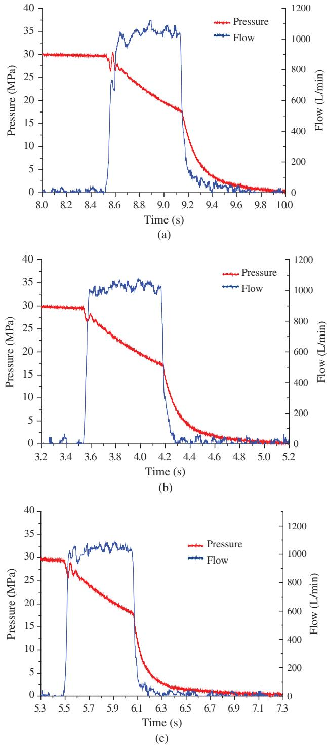
**Figure 9:** Impact characteristics for different pilot valve cores. (a) 30°, (b) 45° and (c) 60°
