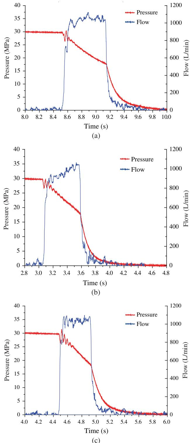
**Figure 11:** Impact characteristics for different flow passage areas. (a) Flow passage area of  $21.6 \text{ mm}^2$ , (b) Flow passage area of  $31.2 \text{ mm}^2$  and (c) Flow passage area of  $36 \text{ mm}^2$
