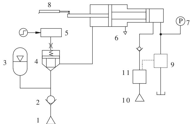
**Figure 7:** Diagram showing the test system. 1. Oil source, 2. One-way valve, 3. Accumulator, 4. Cartridge valves, 5. Pilot valve, 6. Pressure cylinder, 7. Pressure sensor, 8. Displacement sensors, 9. Hydraulic one-way valve, 10. Water pump station and 11. Directional valve
