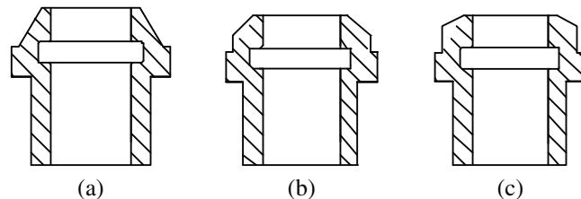
**Figure 4:** Pilot valve core for different cone angles. (a)  $30^\circ$ , (b)  $45^\circ$  and (c)  $60^\circ$
