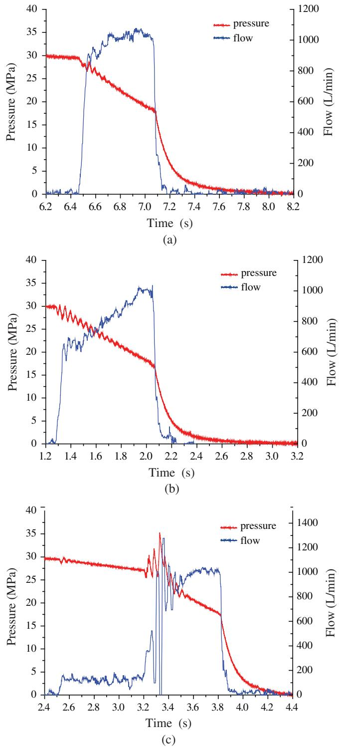
**Figure 10:** Impact characteristics for different main valve cores. (a) Main valve core I. (b) Main valve core II and (c) Main valve core III
