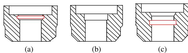
**Figure 5:** Different main valve cores. (a) Main valve core I, (b) Main valve core II and (c) Main valve core III
