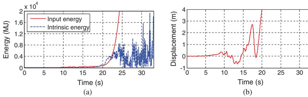
**Figure 8:** The effective energy and the top displacement time histories under EQ2a. (a) Effective energy time histories and (b) Displacement time history
