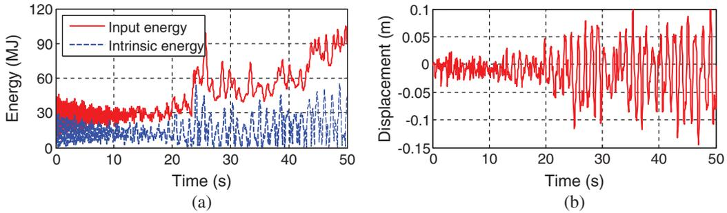
**Figure 5:** The effective energy and the top displacement time histories under EQ1. (a) Effective energy time histories and (b) Displacement time history
