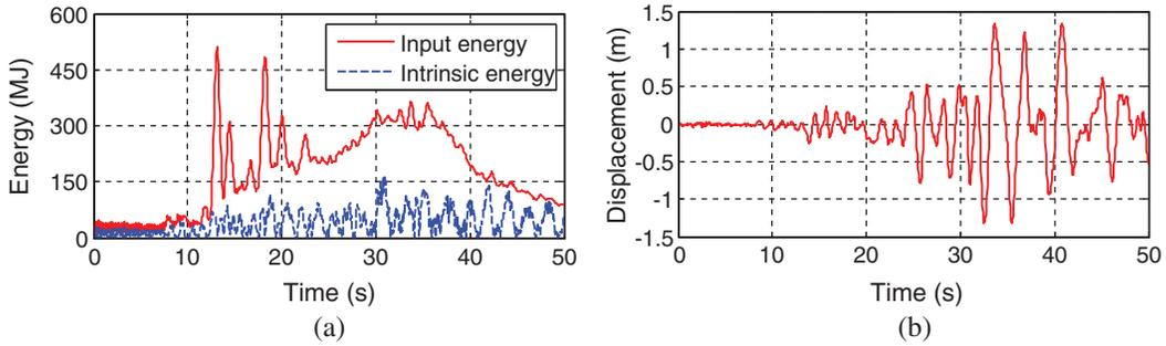
**Figure 11:** The effective energy and the top displacement time histories under EQ1b. (a) Effective energy time histories and (b) Displacement time history
