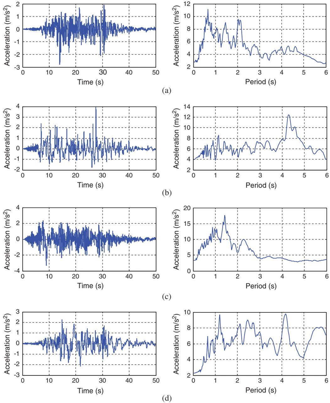
**Figure 3:** The acceleration time histories and response spectra of Chi Chi earthquake. (a) EQ1: TCU049EW (b) EQ2: TCU065EW (c) EQ3: TCU075EW and (d) EQ4: TCU087NS
