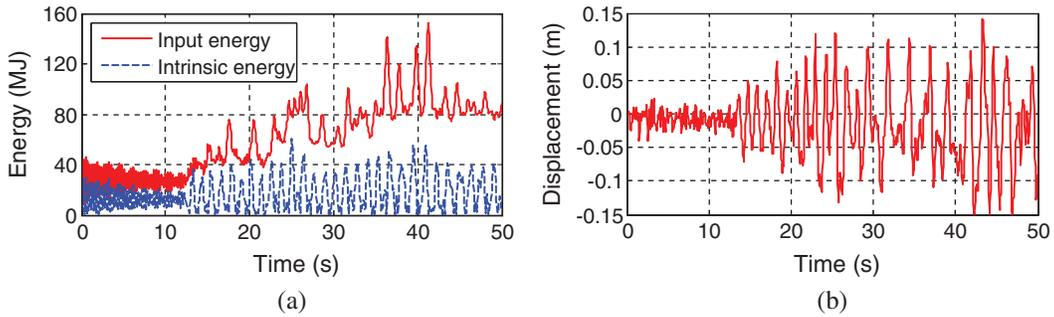
**Figure 6:** The effective energy and the top displacement time histories under EQ2. (a) Effective energy time histories and (b) Displacement time history
