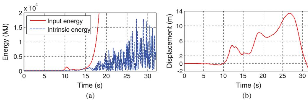
**Figure 13:** The effective energy and the top displacement time histories under EQ3b. (a) Effective energy time histories and (b) Displacement time history
