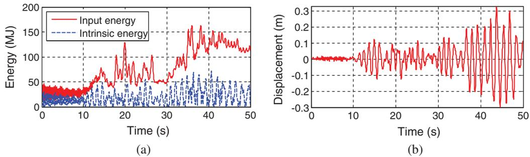
**Figure 10:** The effective energy and the top displacement time histories under EQ4a. (a) Effective energy time histories and (b) Displacement time history
