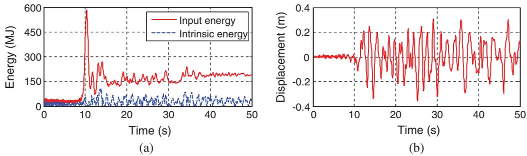
**Figure 9:** The effective energy and the top displacement time histories under EQ3a. (a) Effective energy time histories and (b) Displacement time history
