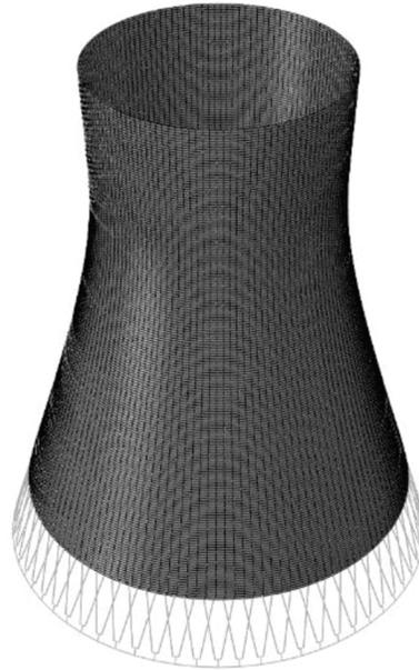
**Figure 2:** FE model of the cooling tower
