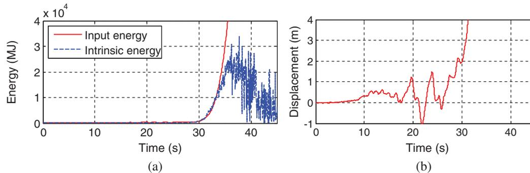
**Figure 14:** The effective energy and the top displacement time histories under EQ4b. (a) Effective energy time histories and (b) Displacement time history
