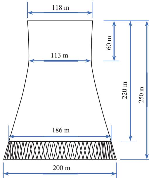
**Figure 1:** Schematic of the cooling tower
