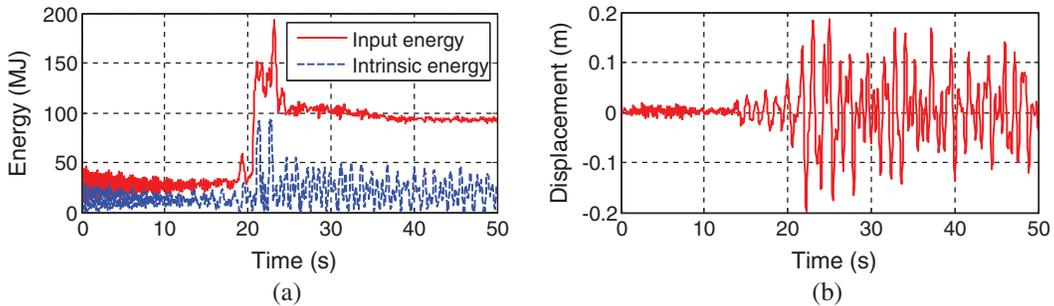
**Figure 7:** The effective energy and the top displacement time histories under EQ1a. (a) Effective energy time histories and (b) Displacement time history
