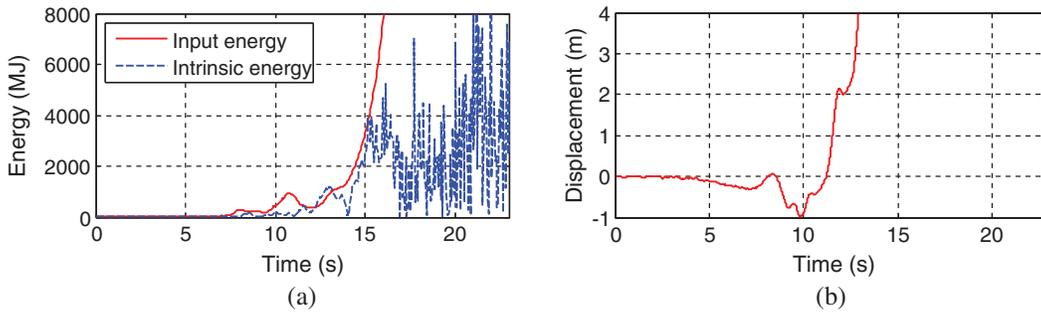
**Figure 12:** The effective energy and the top displacement time histories under EQ2b. (a) Effective energy time histories and (b) Displacement time history
