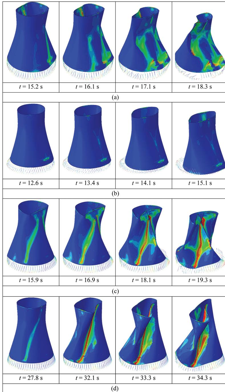
**Figure 4:** The seismic damage processes and collapse modes of the cooling tower. (a) Damage phases under EQ2a: TCU065EW (two times EQ2) (b) Damage phases under EQ2b: TCU065EW (three times EQ2) (c) Damage phases under EQ3b: TCU075EW (three times EQ3) and (d) Damage phases under EQ4b: TCU087NS (three times EQ4)
