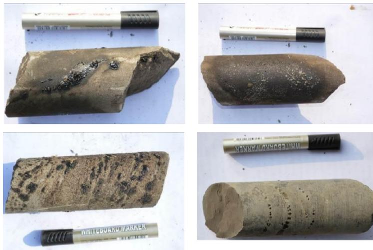
**Figure 5:** Oil patch phenomenon of drill core
