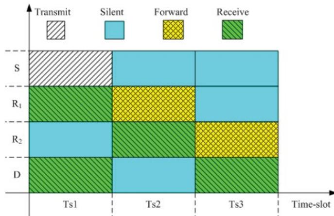
**Figure 2:** Transmission process of ICS scheme
