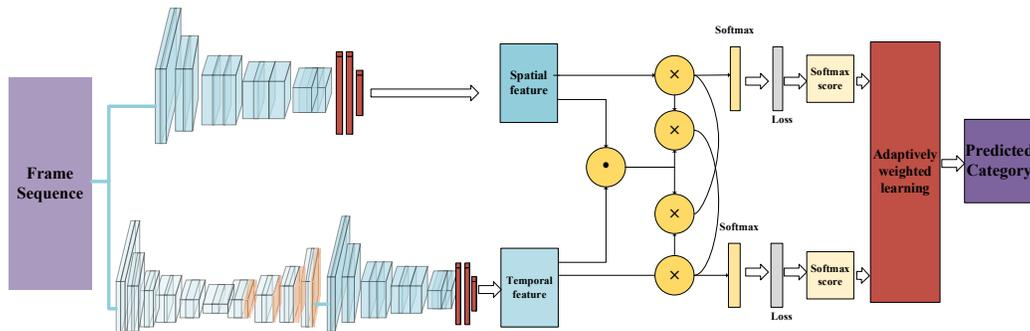
**Figure 2:** The proposed HTSC method consists of two parts: (1) hidden two-stream model learns from the frame sequence to spatial (static) features and temporal (motion) features. (2) collaborative learning model uses the complementarity of motion information and static information to optimize the motion features and static features, which improves the accuracy of action recognition
