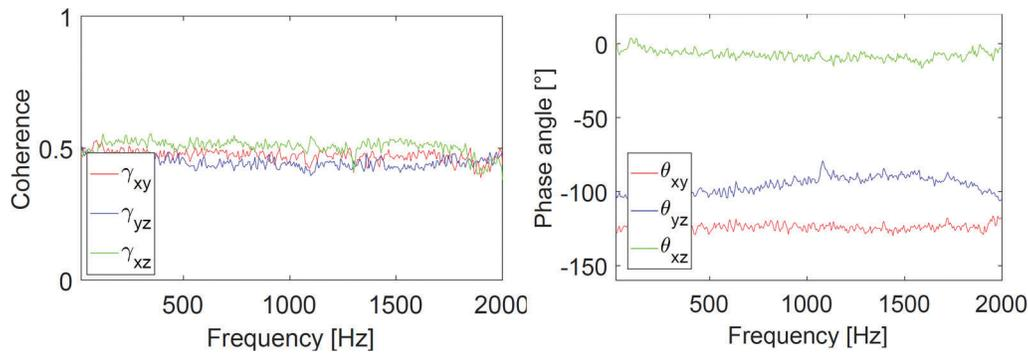
**Figure 12:** Phase and coherence output for input phases  $-120^\circ$ ,  $-120^\circ$ ,  $0^\circ$  and input coherences of 0.5
