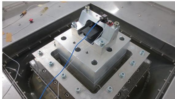
**Figure 11:** Specimen mounted on block with frame setup, control on top
