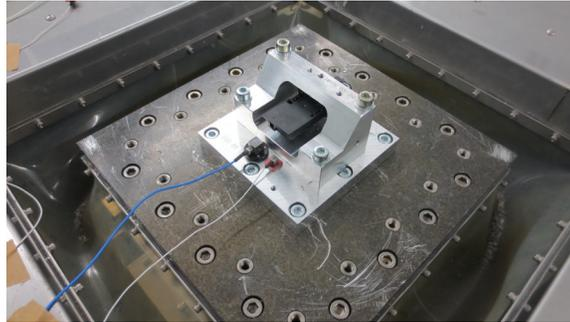
**Figure 8:** Specimen mounted directly on shaker plate, control at bottom
