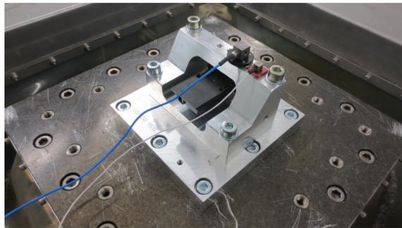
**Figure 9:** Specimen mounted directly on shaker plate, control on top
