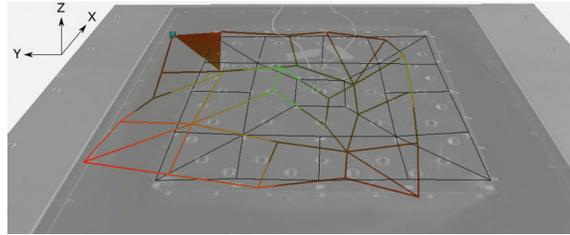
**Figure 4:** Laser vibrometry of second bending mode at around 1850 Hz
