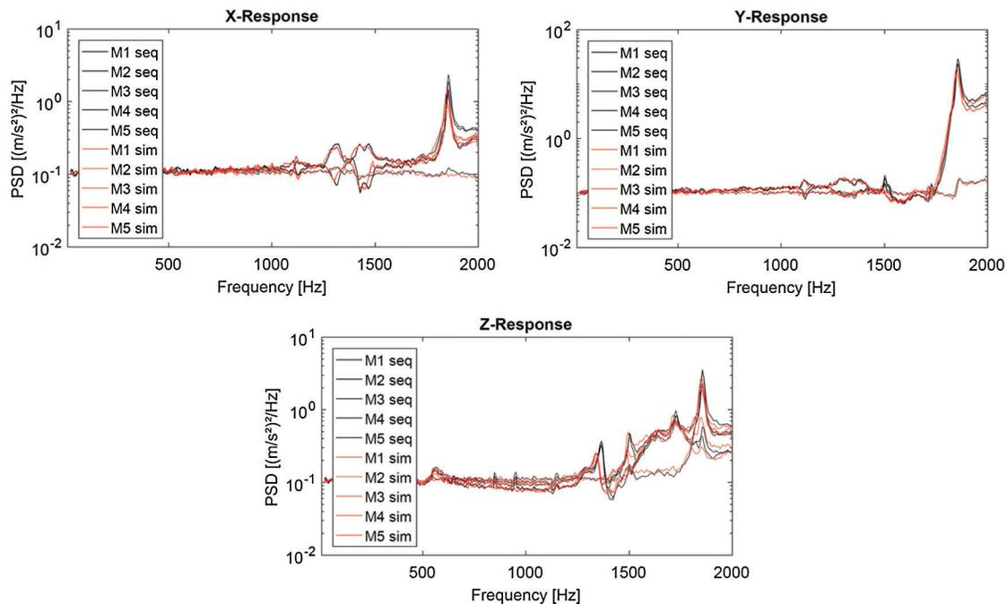
**Figure 3:** Simultaneous and sequential responses in X-,Y- and Z-direction
