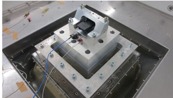
**Figure 10:** Specimen mounted on block with frame setup, control at bottom
