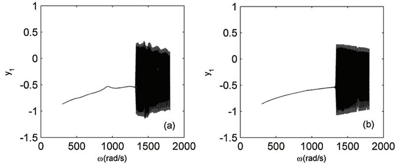
**Figure 4:** Bifurcation diagram of  $y_1$  degree of freedom: (a) the original system (b) the reduced system
