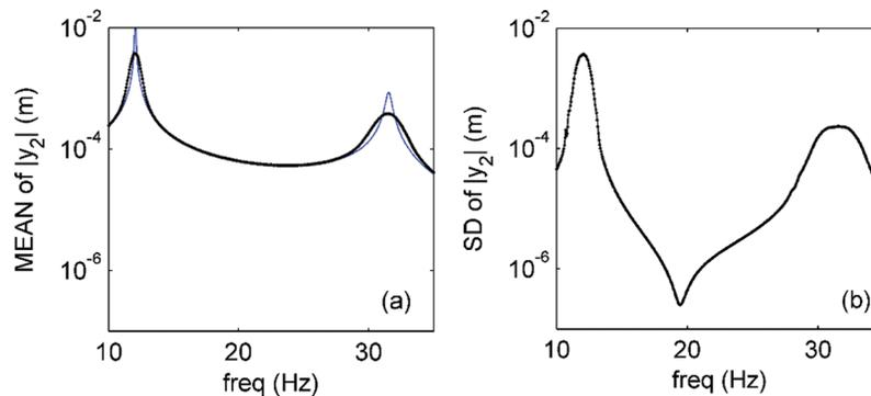
**Figure 6:** Amplitude-frequency curve of the deterministic system (blue), 10000 samples of MCS method (black): (a) first moment of  $y_2$  (b) second moment of  $y_2$
