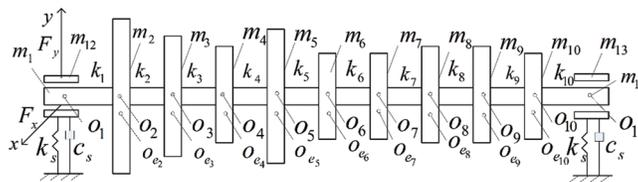
Figure 1: 24-DOF rotor model with looseness at both ends
