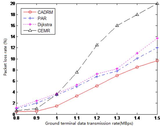
**Figure 3:** Packet loss rate under different transmission rates
