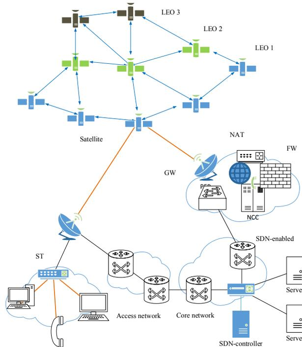
**Figure 2:** Satellite network framework based on SDN
