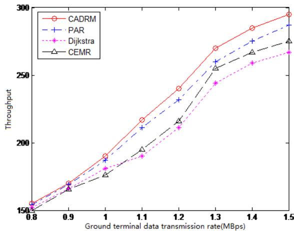
**Figure 4:** Throughput at different transmission rates
