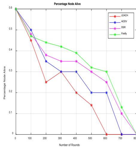
Figure 7: Percentage of the alive node inside the network
