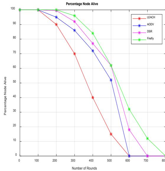
Figure 6: Percentage of an alive node outside the network
