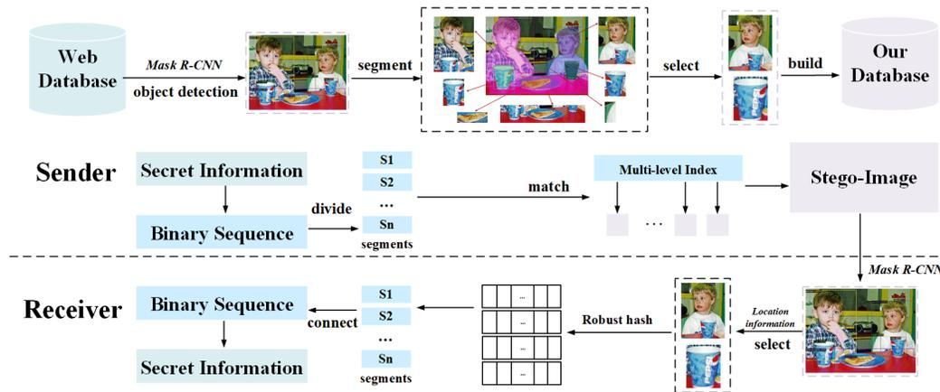
Figure 7: Coverless image steganography based on image segmentation
