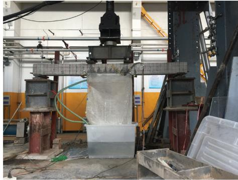
**Figure 3:** Corrosion fatigue coupling test method
