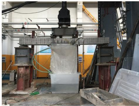
**Figure 3:** Corrosion fatigue coupling test method
