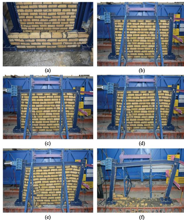
**Figure 9:** The CF-2 frame. (a) How the bracing rebars are added. (b) View of the frame before loading. (c) 5% of drift. (d) 10% of drift. (e) 15% of drift. (f) Final deformation of the frame
