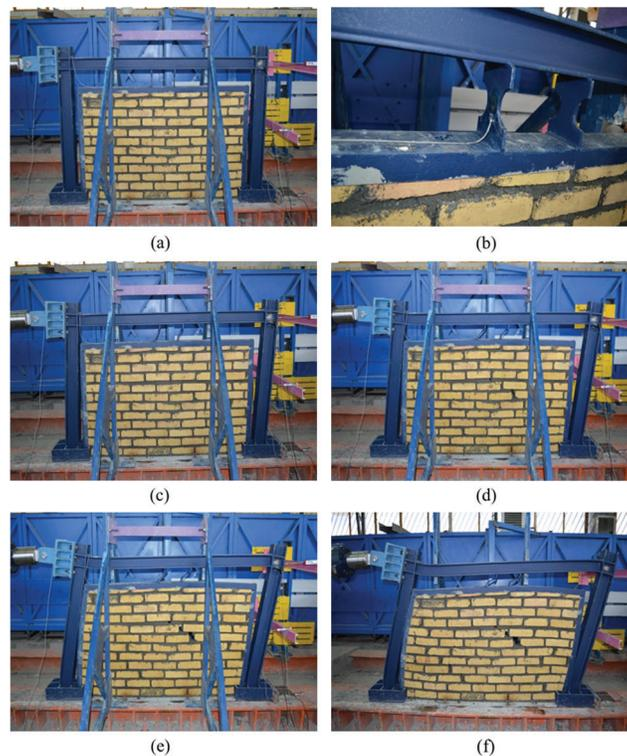
**Figure 11:** The CF-3 frame. (a) View of the frame before loading. (b) Connecting plates. (c) 5% of drift. (d) 10% of drift. (e) 15% of drift. (f) Final deformation of the frame
