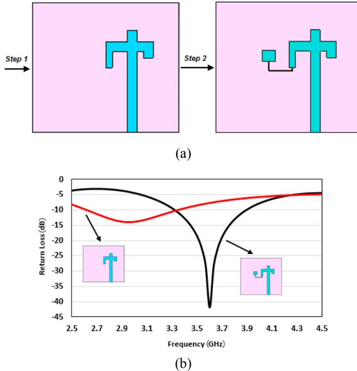
**Figure 2:** Design layout and return loss comparison (a) Design evaluation steps (b) Return loss comparison of the design evaluation steps
