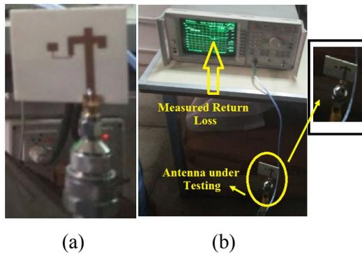
**Figure 9:** Fabricated antenna (a) Connected with a connector (b) Under testing
