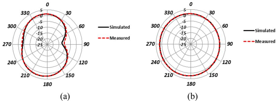
**Figure 10:** Simulated and measured results (a) H-plane (b) E-plane
