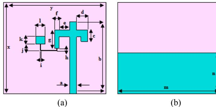
**Figure 1:** Geometry of antenna (a) Front view (b) Back view
