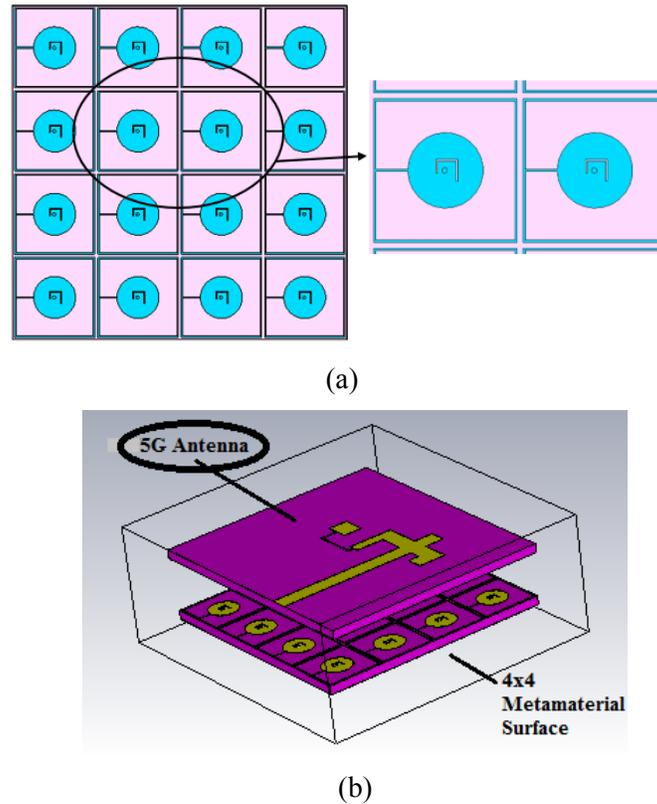
**Figure 5:** (a) 4×4 metamaterial surface (b) Antenna incorporated with a meta-surface
