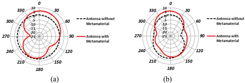
**Figure 7:** Radiation pattern (2D) (a) E plane (b) H plane
