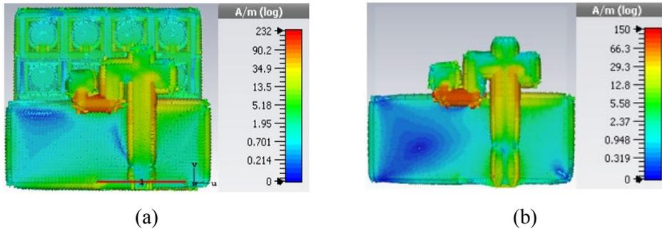
**Figure 8:** Surface current distribution (a) Metamaterial-based antenna (b) Antenna without metamaterial surface
