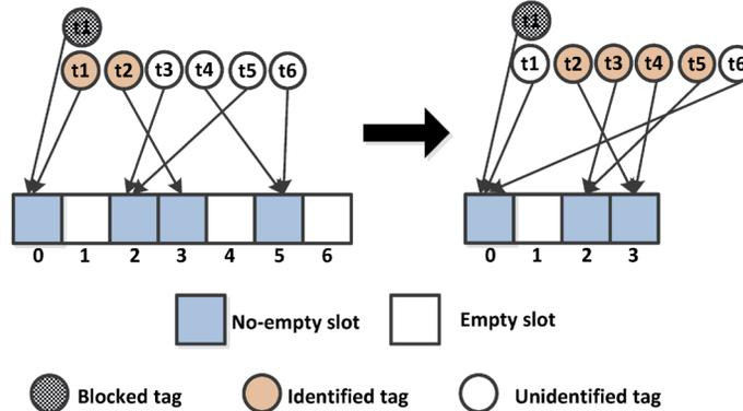
Figure 2: An example of identifying more tags with less time slots
