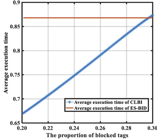
**Figure 5:** The average execution time for verifying a tag with respect to  $p$
