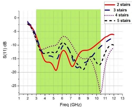
**Figure 6:** Reflection coefficient with different number of stairs in the ground plane
