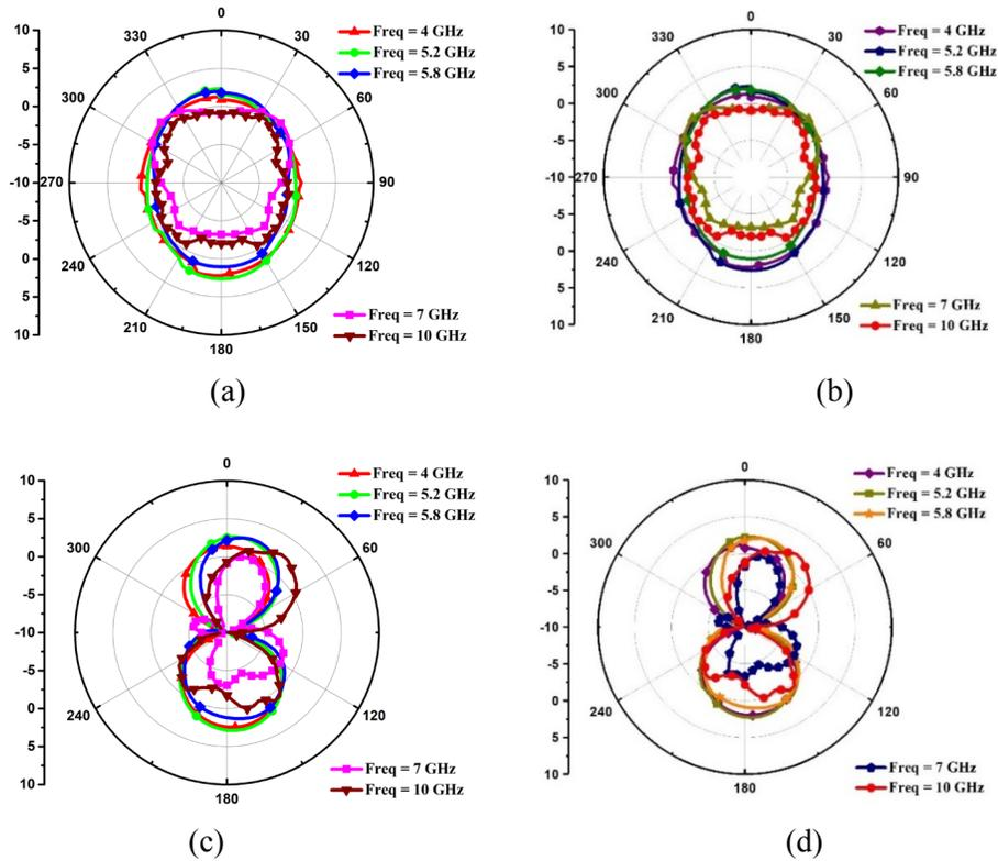
**Figure 9:** (a) Simulated YZ or H plane radiation pattern (b) Measured YZ or H plane radiation pattern (c) Simulated XZ or E plane radiation pattern (d) Measured XZ or E plane radiation pattern
