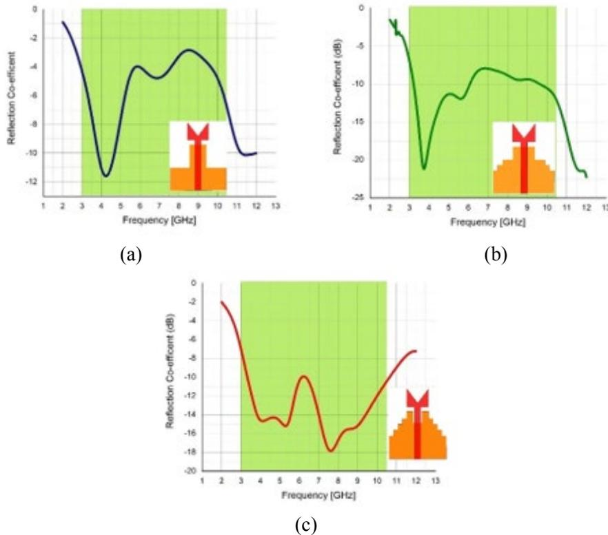
**Figure 3:** Reflection coefficient (a) Geometry-1 (b) Geometry-2 (c) Geometry-3
