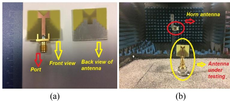
**Figure 7:** (a) Fabricated prototype of antenna (b) Antenna for testing in anechoic chamber
