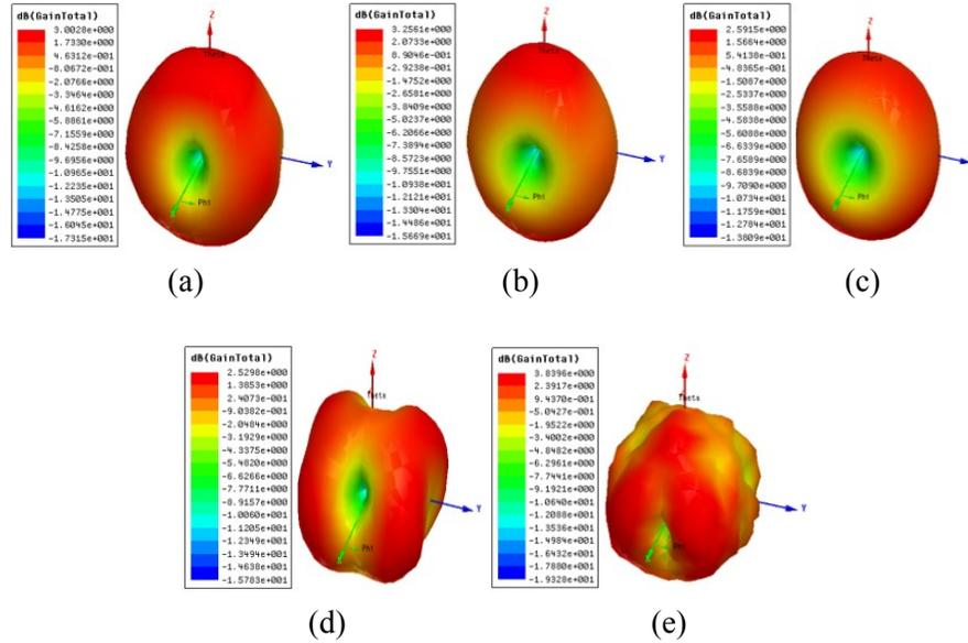
**Figure 11:** 3D gain patterns of the designed Antenna at the desired frequencies of (a) 5.8 GHz (b) 5.2 GHz (c) 4.0 GHz (d) 7.0 GHz (e) 10.0 GHz
