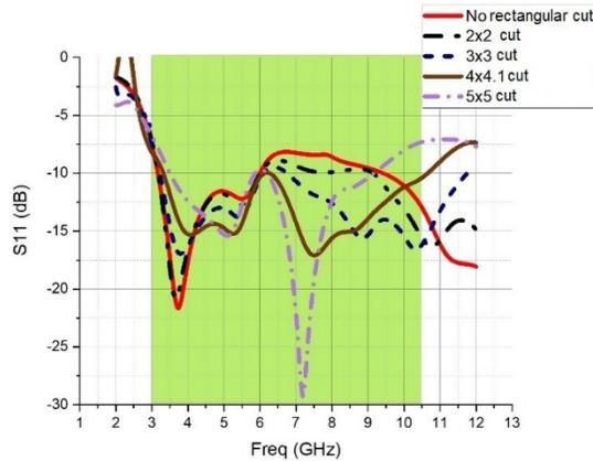
**Figure 5:** Reflection coefficient with different values of rectangular cut in the middle of top staircase
