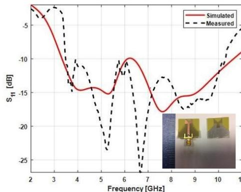
**Figure 8:** Simulated and measured reflection coefficient comparison
