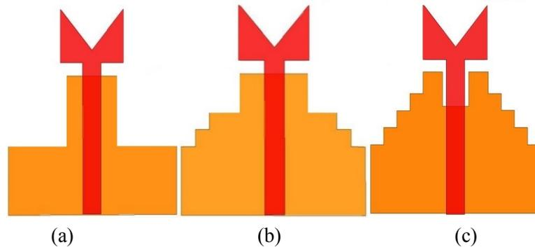
**Figure 2:** Proposed antenna evolution (a) Geometry-1 (b) Geometry-2 (c) Geometry-3
