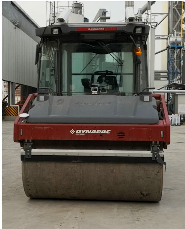
Figure 9: Dynapac CC6200 double drum vibratory roller
