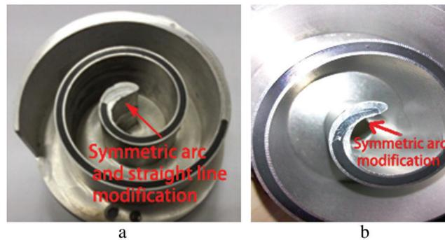
**Figure 2:** Modifications of the end profile of the dynamic scroll disk. a) Symmetrical-arc and straight-line modification. b) Symmetric arc modification
