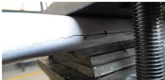
**Figure 11:** Crack occurred at root portion of solid blade (side view)
