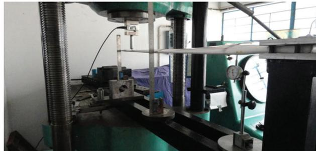
**Figure 10:** Load deflection test setup used when load is applied at tip of fabricated blade
