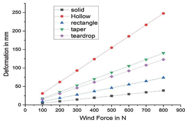
**Figure 6:** Variation of deformation with respect to wind force on different blades
