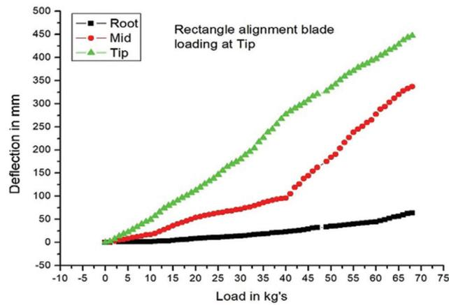
Figure 15: Load deflection test results for R-22-Rectangular alignment blade
