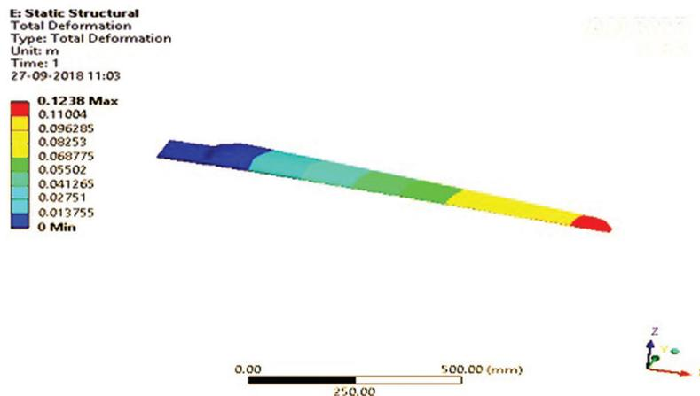
**Figure 4:** Total deformation of SWT Blade loaded at the tip
