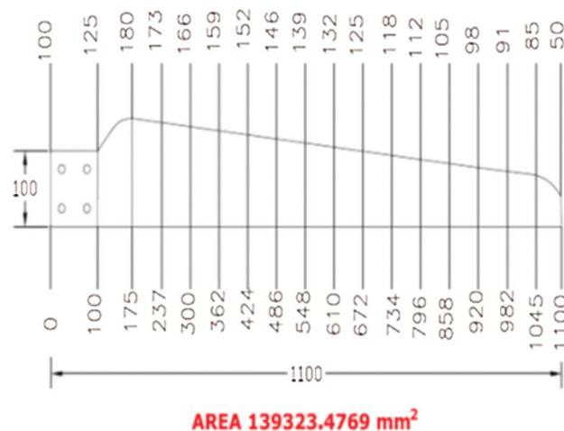
**Figure 2:** Two dimensional model of a small wind turbine (SWT) blade [20]
