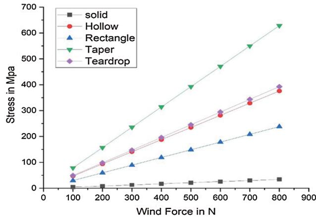
**Figure 7:** Stress variation at different wind forces on different blades
