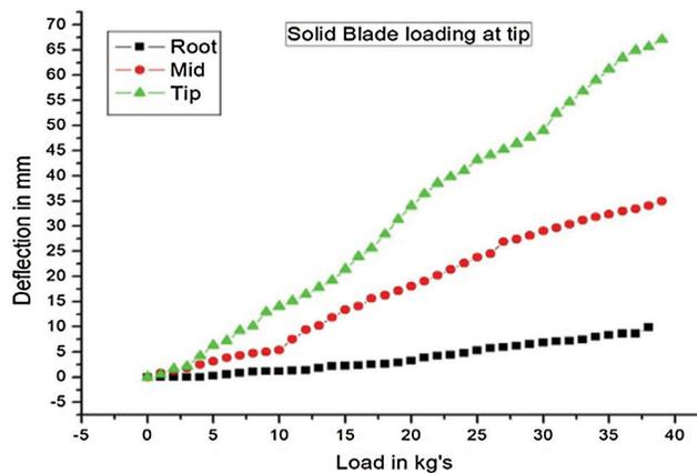
**Figure 13:** Load deflection test results for R-22-Solid blade
