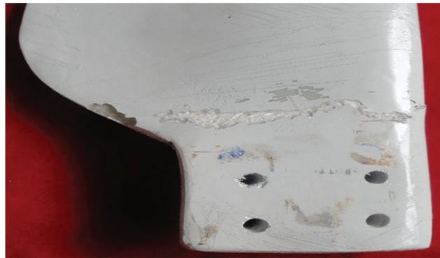
**Figure 12:** Crack occurred at root portion of rectangle alignment blade (top view)
