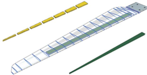
**Figure 3:** CAD model of a SWT blade with various alignments at inner core
