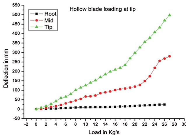
**Figure 14:** Load deflection test results for R-22-Hollow blade
