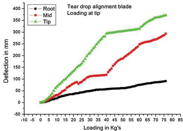
Figure 17: Load deflection test results for R-22-Teardrop alignment blade
