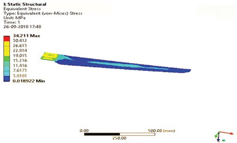
**Figure 5:** Stress distribution of SWT blade loaded at the tip
