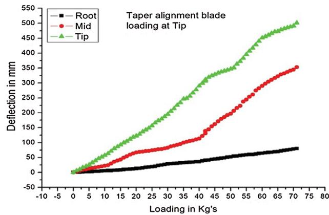
Figure 16: Load deflection test results for R-22-Taper alignment blade
