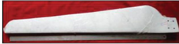
**Figure 9:** Fabricated model of NACA 63415 aerofoil blade
