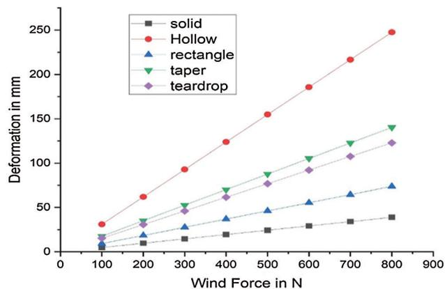
**Figure 6:** Variation of deformation with respect to wind force on different blades
