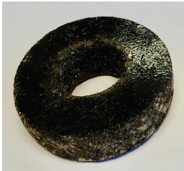
Figure 7: Digital image of the grinding wheel based on TFUG resin matrix
