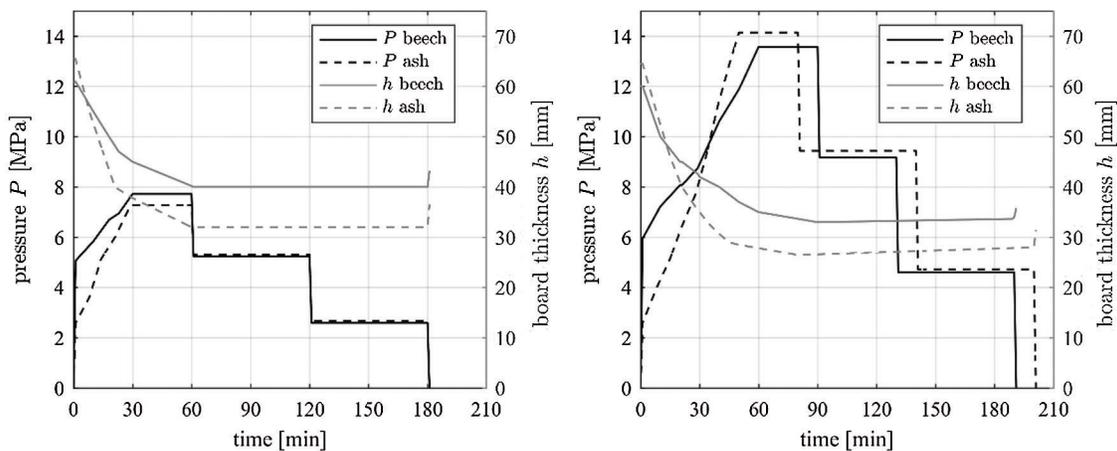
**Figure 1:** Pressing procedure and corresponding thickness reduction for beech and ash densified to 1.0 t/m<sup>3</sup> (left) and 1.2 t/m<sup>3</sup> (right)
