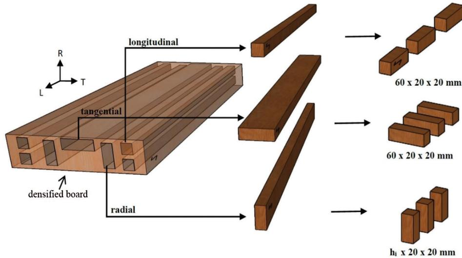
**Figure 3:** Cutting of compression test specimens from the boards
