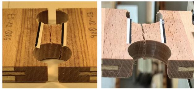
**Figure 14:** Failure pattern for tension in radial (left) and tangential (right) direction
