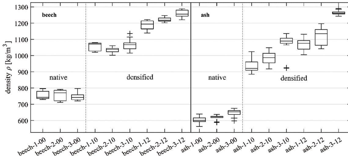
**Figure 5:** Obtained densities after densification as boxplot diagram. Whiskers display values within  $1.5 \times$  the interquartile range, values out of this range are displayed as outliers in form of a cross. Board labels: wood type—No. of board—densification level (00 = native, 10 =  $1.0 \text{ t/m}^3$  and 12 =  $1.2 \text{ t/m}^3$  target density)
