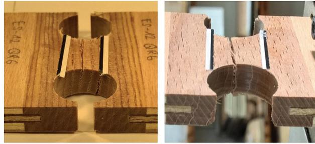
**Figure 14:** Failure pattern for tension in radial (left) and tangential (right) direction
