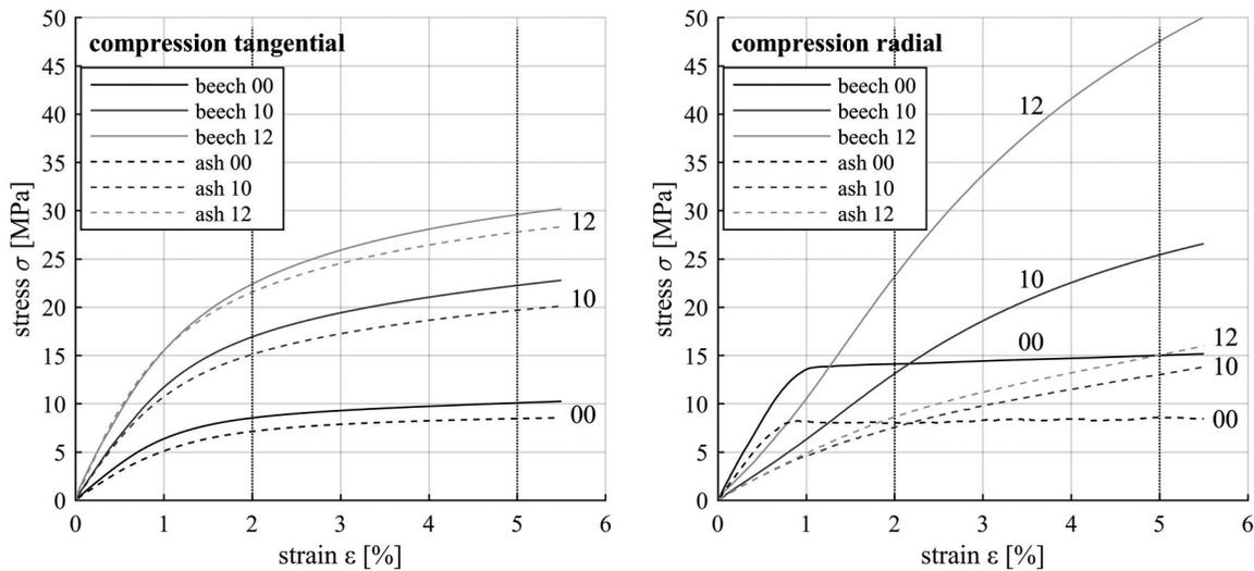
**Figure 8:** Stress-strain diagrams for compression perpendicular to the grain. Mean curves for densification levels 00 (native), 10 (1.0 t/m<sup>3</sup>) and 12 (1.2 t/m<sup>3</sup>)
