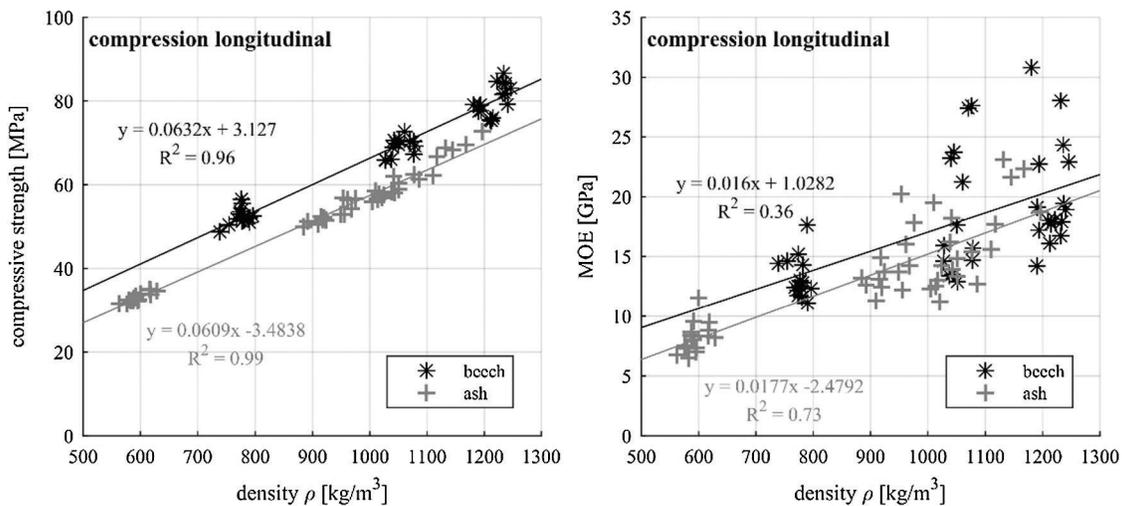
**Figure 6:** Compression strength (left) and MOE (right) parallel to the fibre (longitudinal) in relation to the density
