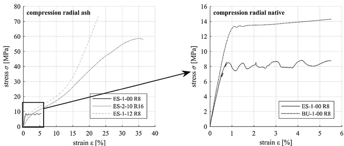
**Figure 10:** Stress-strain curves of individual specimens from the compression tests in radial direction. Comparison of the three density levels of ash (left), enlarged for the native specimen and compared with native beech (right)
