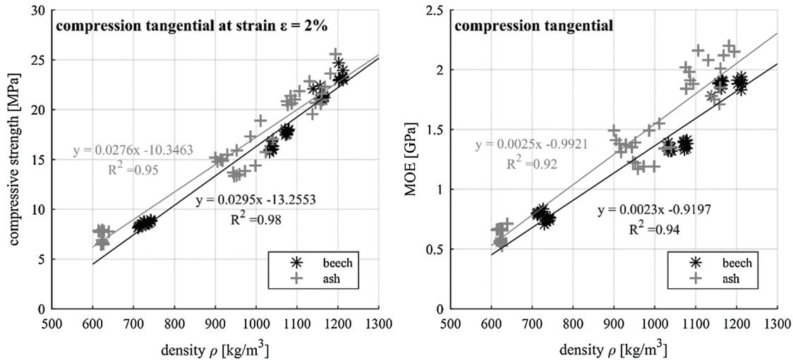
**Figure 7:** Compressive strength (left) and MOE (right) in tangential direction in relation to the density
