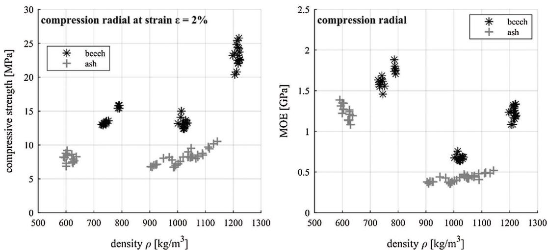
**Figure 9:** Compressive strength at 2% strain and MOE radial in relation to the density
