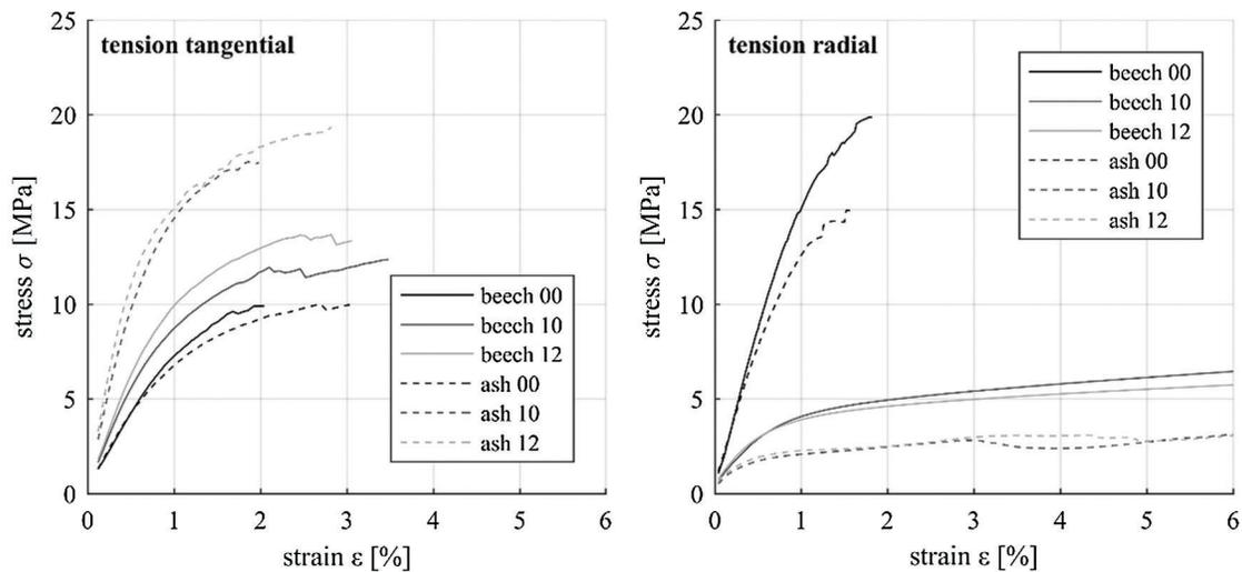
**Figure 11:** Stress-strain diagrams for tension perpendicular to the grain. Mean values for densification levels 00 (native), 10 (1.0 t/m<sup>3</sup>) and 12 (1.2 t/m<sup>3</sup>)
