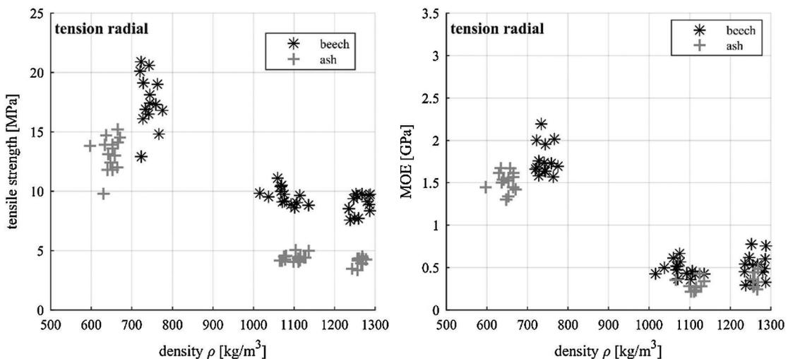
**Figure 13:** Material behaviour under tension in radial direction in relation to the density
