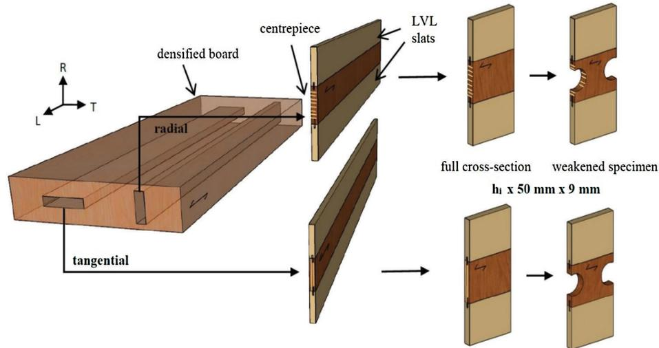
**Figure 4:** Cutting of radial and tangential tension specimens
