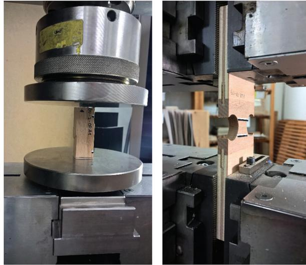
**Figure 2:** Test setup for compression and tension tests. Left: Beech specimen after compression test in fibre direction, right: Beech specimen during tensile test in tangential direction
