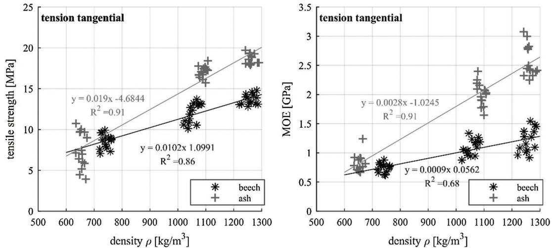
**Figure 12:** Tensile strength (left) and MOE (right) in tangential direction in relation to the density
