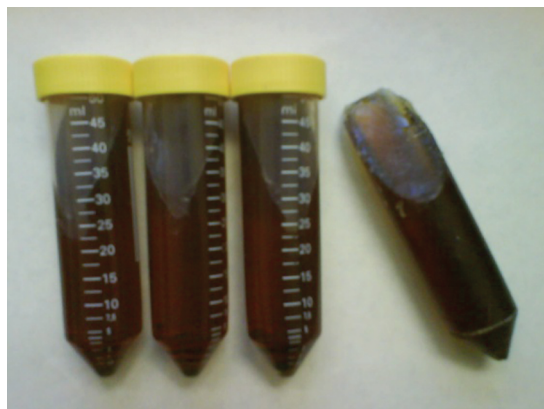
Figure 3: PET ampoules ( D_{in} = 25.4 mm) with hardened, monolithic petrochemical PUR and a PUR rod
