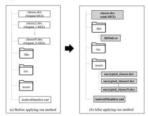
Figure 5. Structure of APK files before/after Packing.
