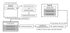
Figure 3. Execution Flow of Multidex APK.
