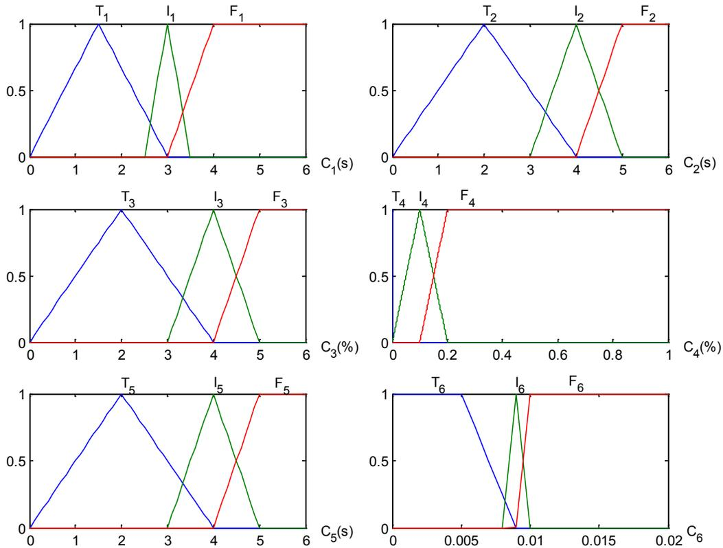
**Figure 2.** The membership functions of six transient state characteristics. C1: rising time (s), C2: settling time (s), C3: overshoot ratio (%), C4: undershoot ratio (%), C5: peak time (s), and C6: steady-state error.
