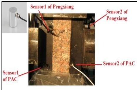
Figure 6. Sensors and their parameters.
