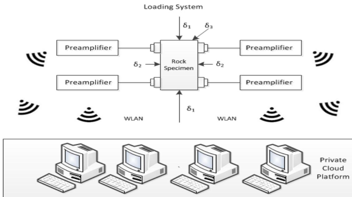
Figure 3. Acoustic emission data collection cloud platform.
