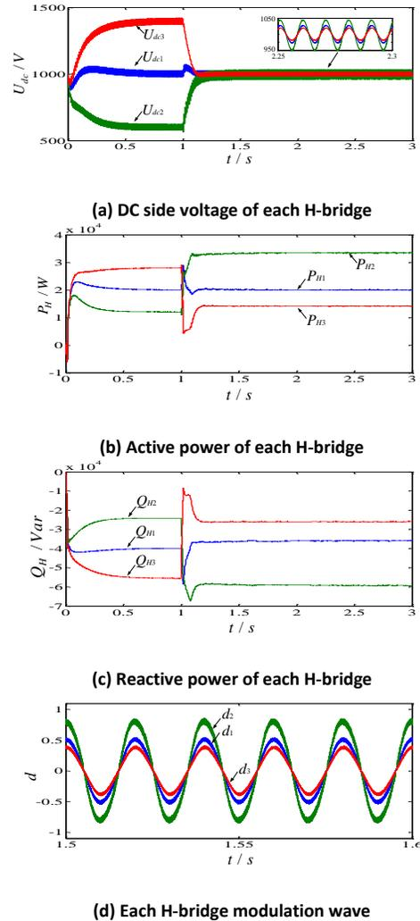
**Figure 11.** Waveforms under the traditional method
