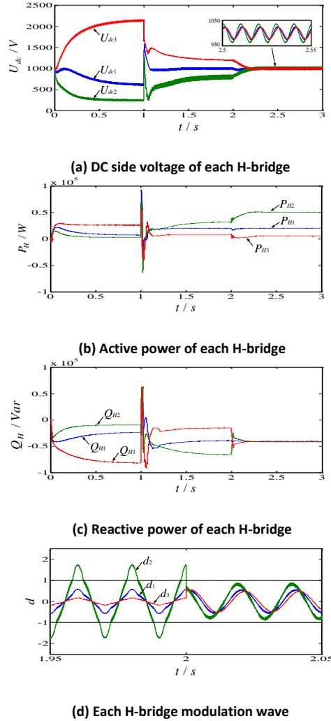
Figure 13. Comparison of two control methods under large load imbalance
