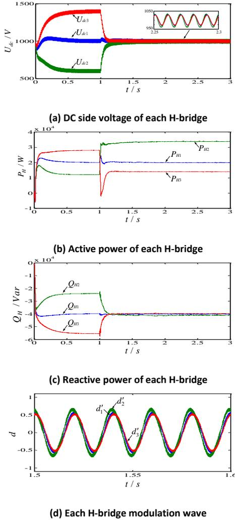
Figure 12. Waveforms under the proposed method
