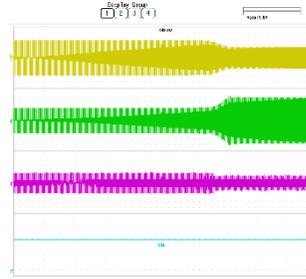
(c) Waveform under the condition of voltage sag
