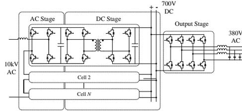
Figure 1. Circuit topology of single-phase SST
