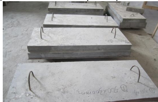
(d): Before the final solidification of concrete, the steel plate was removed and slab with precast crack was produced
