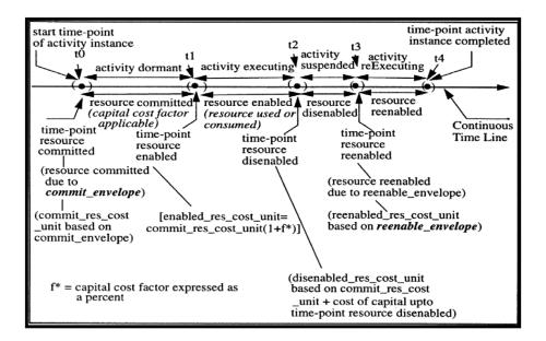
Figure 4. Activity Instance on Continuous Time Line.
