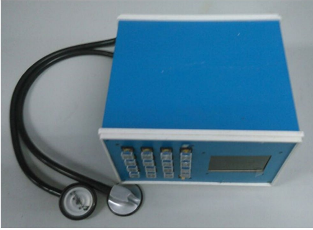
Figure 1. Lung Sound Acquisition Device Made by Our Team.
