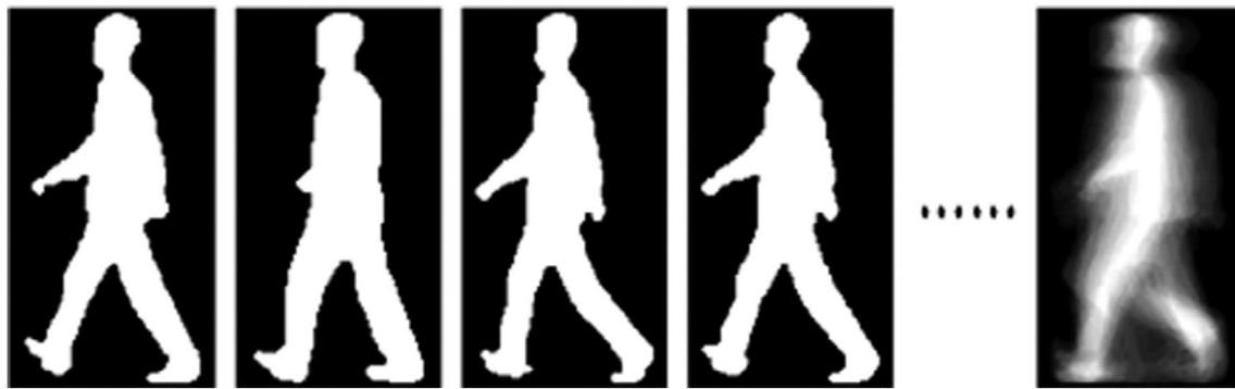
Figure 4. The post-process image from a series of gait-energy image processing.
