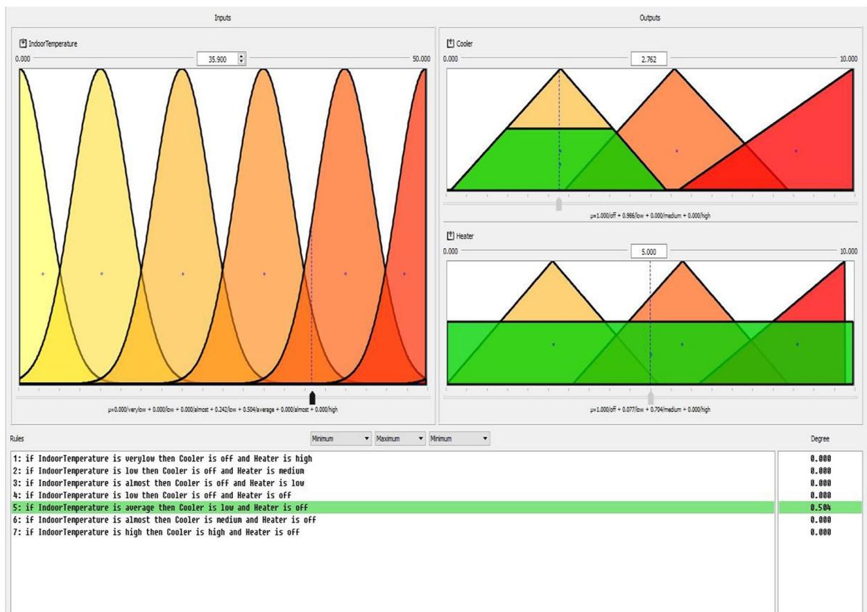
**Figure 3.** Implementation of the Cooler/heater System Using Fuzzylite.
