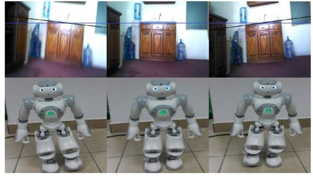
Figure 6. Motivation for a Rotated BRIEF Vocabulary. As the Humanoid Robot Walks, the Images Captured by the Onboard Camera are Rotated with Respect to the Optical Axis.
