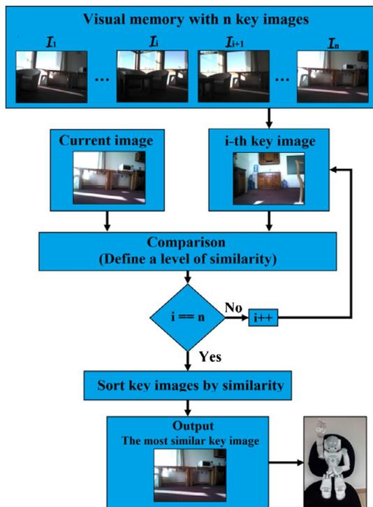
Figure 1. General Diagram of the Appearance-based Localization from a Visual Memory.
