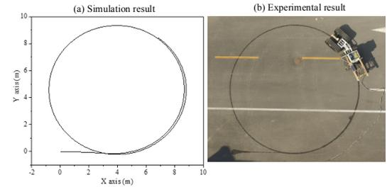
**Figure 3.** Trajectory Comparison of Simulation and Experiment.
