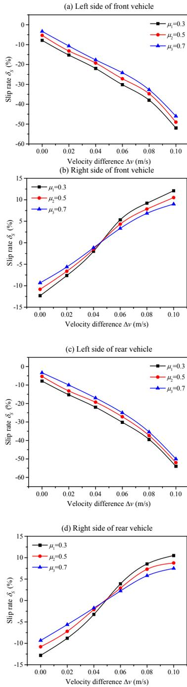
**Figure 19.** Effect of Ground Friction Coefficient and Velocity Difference under  $R_L=9.01$  m.
