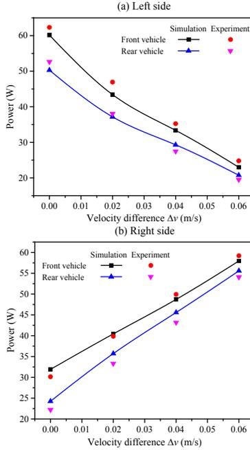
Figure 5. Average Power Comparison of Simulation and Experiment.
