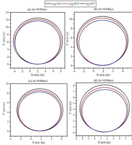
**Figure 14. Effect of Velocity Difference and Ground Friction Coefficient on the Steering Trajectory.**
