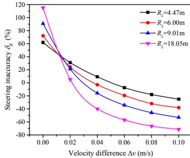
**Figure 10. Effect of Velocity Difference and Theoretical Steering Radius on Steering Inaccuracy.**
