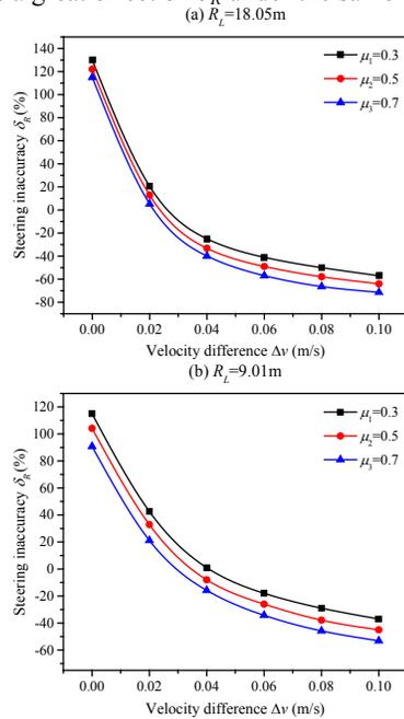
**Figure 17.** Effect of the Theoretical Steering Radius and Ground Friction Coefficient under Different Velocity Difference on Steering Inaccuracy.
