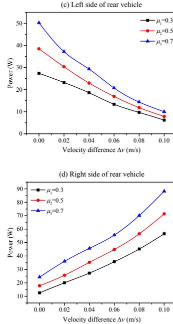
**Figure 12. Effect of Velocity Difference and Ground Friction Coefficient on Driving Power.**
