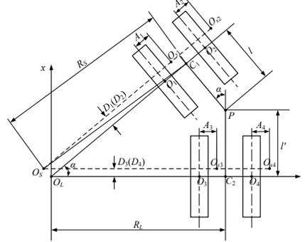
Figure 6. Steering Motion Diagram.
