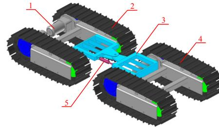
**Figure 1. Virtual Prototype Model of the Articulated Crawler: 1 Drive motor, 2 Rear vehicle, 3 Articulated frame, 4 Front vehicle, and 5 Linear actuator.**
