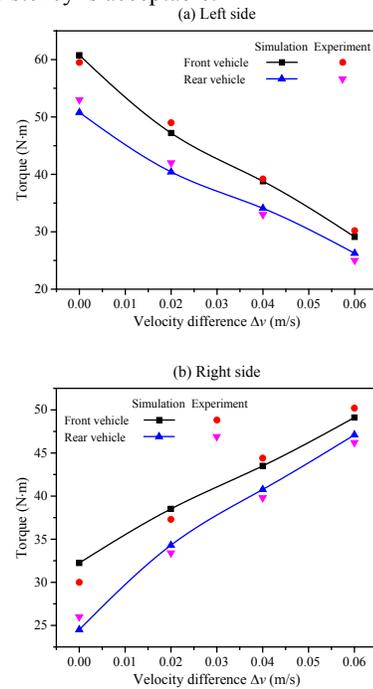
**Figure 4.** Average Torque Comparison of Simulation and Experiment.
