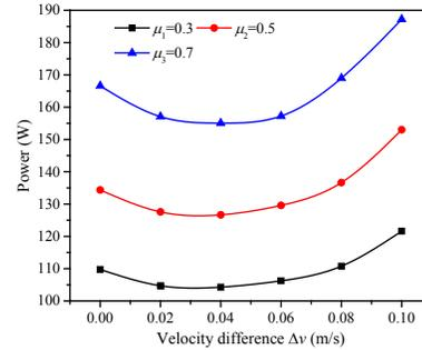
**Figure 13. Effect of Velocity Difference and Ground Friction Coefficient on Total Driving Power.**
