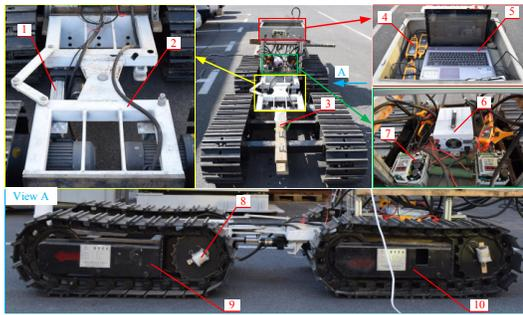
**Figure 2.** Experimental Prototype of the Articulated Vehicle: 1 Linear actuator, 2 Articulated frame, 3 Trajectory drawing device, 4 Frequency meter, 5 Laptop, 6 Stabilized power supply, 7 Frequency converter, 8 Torque sensor, 9 Front vehicle, and 10 Rear vehicle.
