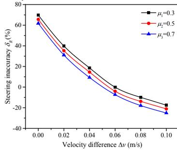
**Figure 15. Effect of Velocity Difference and Ground Friction Coefficient on the Steering Inaccuracy.**
