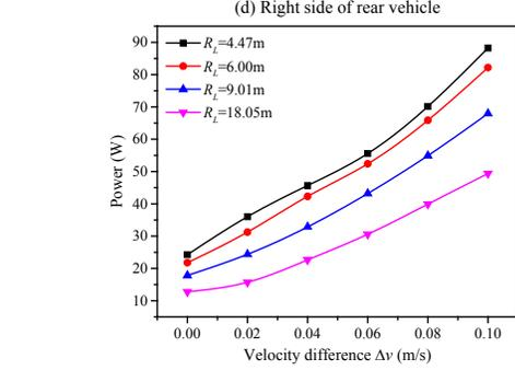
**Figure 7. Effect of Velocity Difference and Theoretical Steering Radius on Driving Power.**
