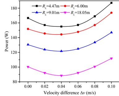
**Figure 8. Effect of Velocity Difference and Theoretical Steering Radius on Total Driving Power.**
