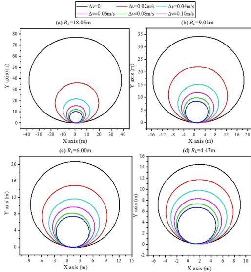
**Figure 9. Effect of Velocity Difference and Theoretical Steering Radius on Steering Trajectory.**
