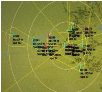
Figure 4. ADS-B Display Information of the Track of Circle and Eight Character Procedures.
