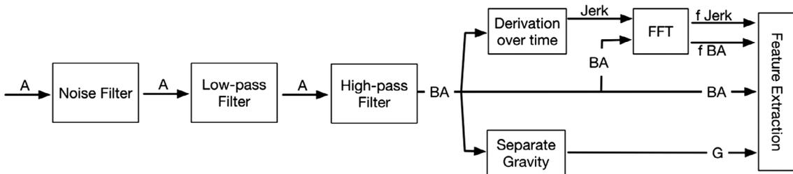
**Figure 2.** Processing of Raw Accelerometer Sensor Readings from Embedded Accelerometer of Smartphone to Generate Body Acceleration Data (BA), Gravity Data (G), Body Acceleration Jerk Data (Jerk), and Body Acceleration Frequency Data (f Jerk and f BA).
