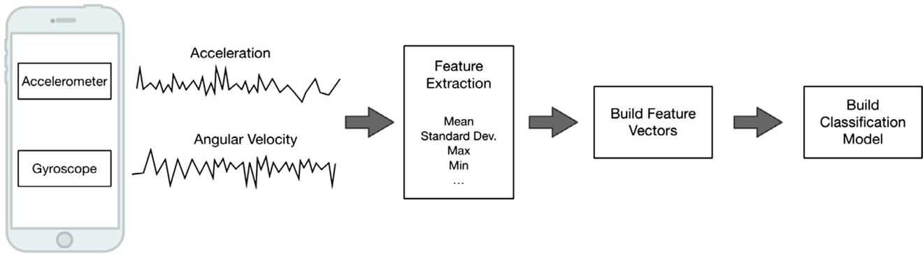
**Figure 1.** The Process of Sampling Acceleration Sensor Readings and Angular Velocity Sensor Readings from the Accelerometer and the Gyroscope Embedded in a Smartphone, Extracting Features, and using the Features to Train a Model for Activity Recognition.
