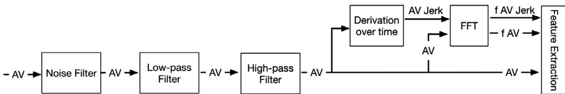
**Figure 3.** Processing of Sensor Readings from Embedded Gyroscope of Smartphone to Generate Angular Velocity Data (AV), Angular Velocity Jerk Data (AV Jerk), and Angular Velocity Frequency Data (f AV and f AV Jerk).
