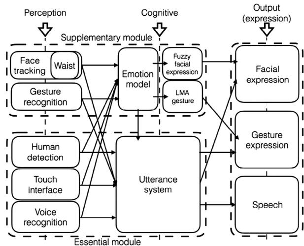
**Figure 13.** Functional Block Diagram of Cognitive System.
