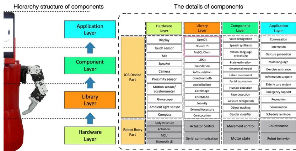
Figure 5. The Modular Architecture Layer of iPhonoid.
