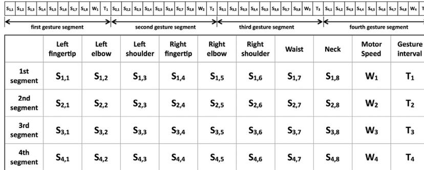
**Figure 9.** Chromosome Structure of Motors for each Feeling in the Robot's Gesture.
