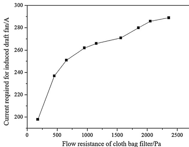
**Figure 7:** Relationship between the flow resistance of the bag filter and the current required by the induced draft fan
