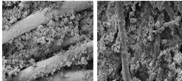
**Figure 5:** Electron microscopy of the windward surface of the filter bag
