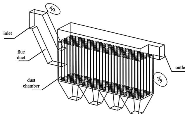
**Figure 1:** Structure diagram of a bag filter
