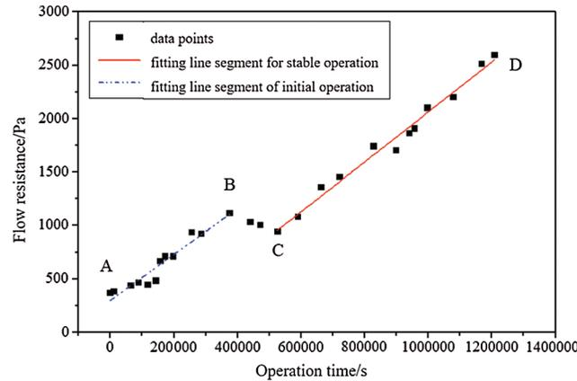
**Figure 3:** Relationship between flow resistance and operation time of the bag filter
