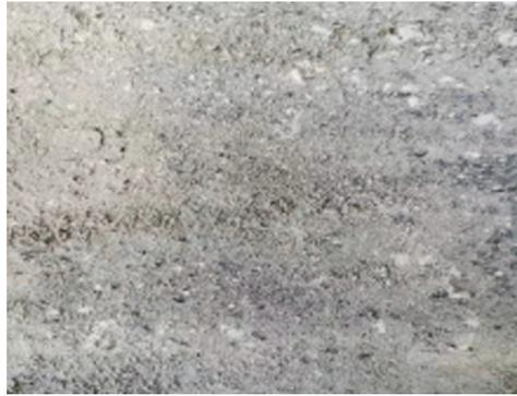
**Figure 4:** Dust layer on the windward side of the filter bag
