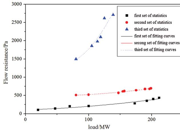
**Figure 6:** Relationship between the boiler load and the flow resistance of the bag filter
