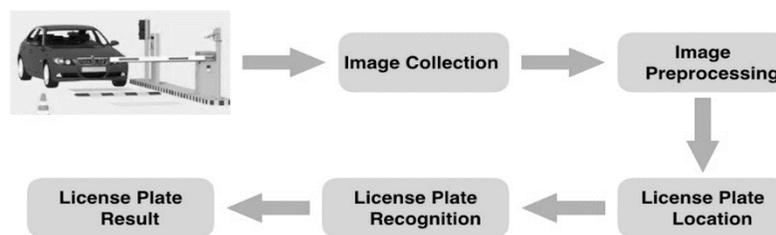
**Figure 1:** License plate recognition process
