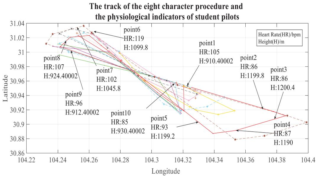
Figure 3 Flight data of the eight character procedure in a domestic flight training institution.
