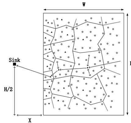
Figure 1. Distribution Map of the Sink and Sensor Node.
