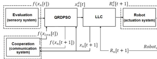
Figure 1. QRDPSO control architecture
