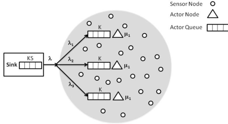
Figure 1 A queuing network model of WSAN.
