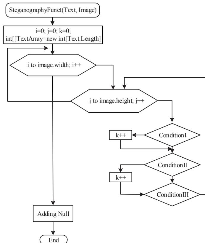
Figure 1 Flow of the enhanced bit substitution algorithm.
