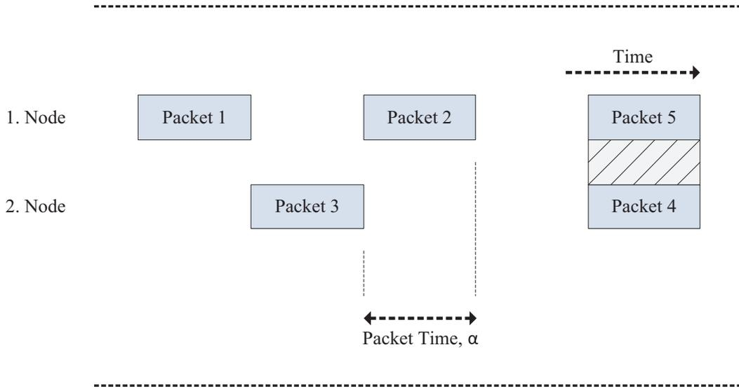
Figure 2 Slotted Aloha technique sample packet transmission
