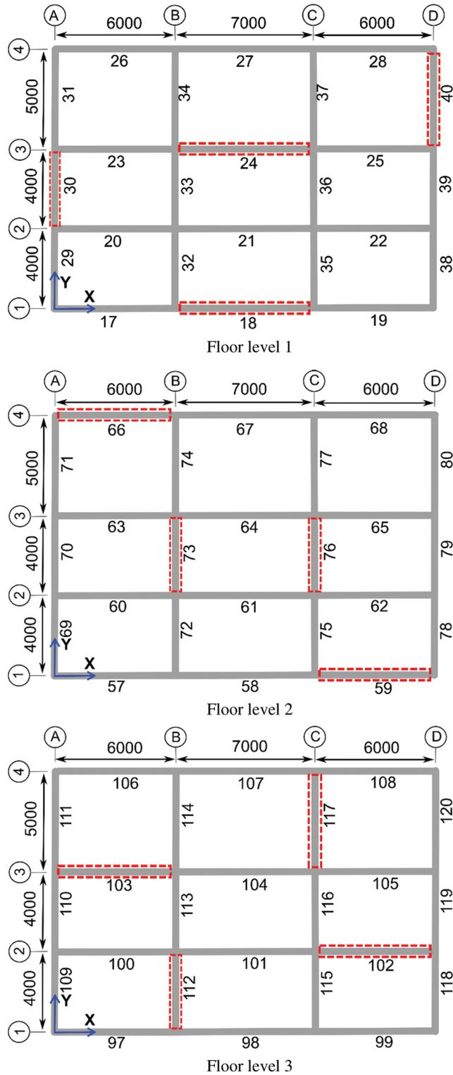
**Figure 6:** Location of elements with damage in levels 1, 2 and 3 (dimensions in mm). Damaged element and ID numbering
