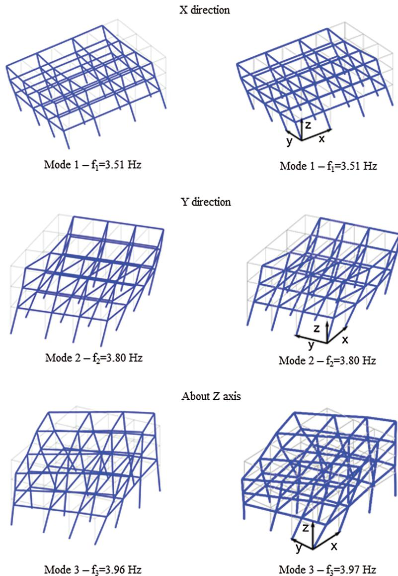
**Figure 10:** Comparison of the first 3 mode shapes of the building without damage calculated using SAP2000<sup>®</sup> (left column) and the proposed dynamic simulation method (right column)
