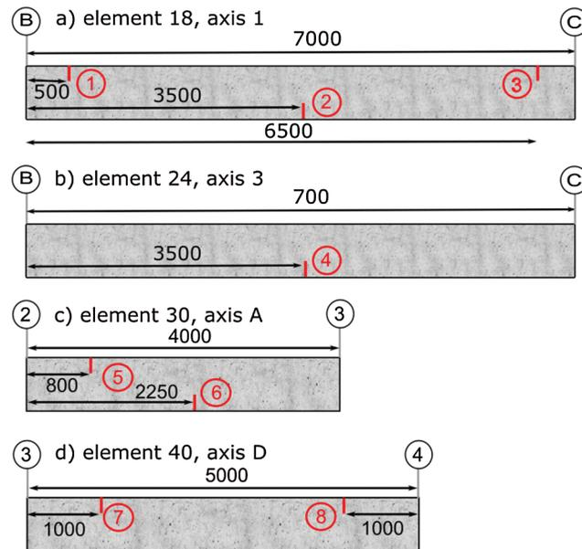
**Figure 7:** Damage location at first level beams (dimensions in mm). a) element 18, axis 1. b) element 24, axis 3. c) element 30, axis A. d) element 40, axis D
