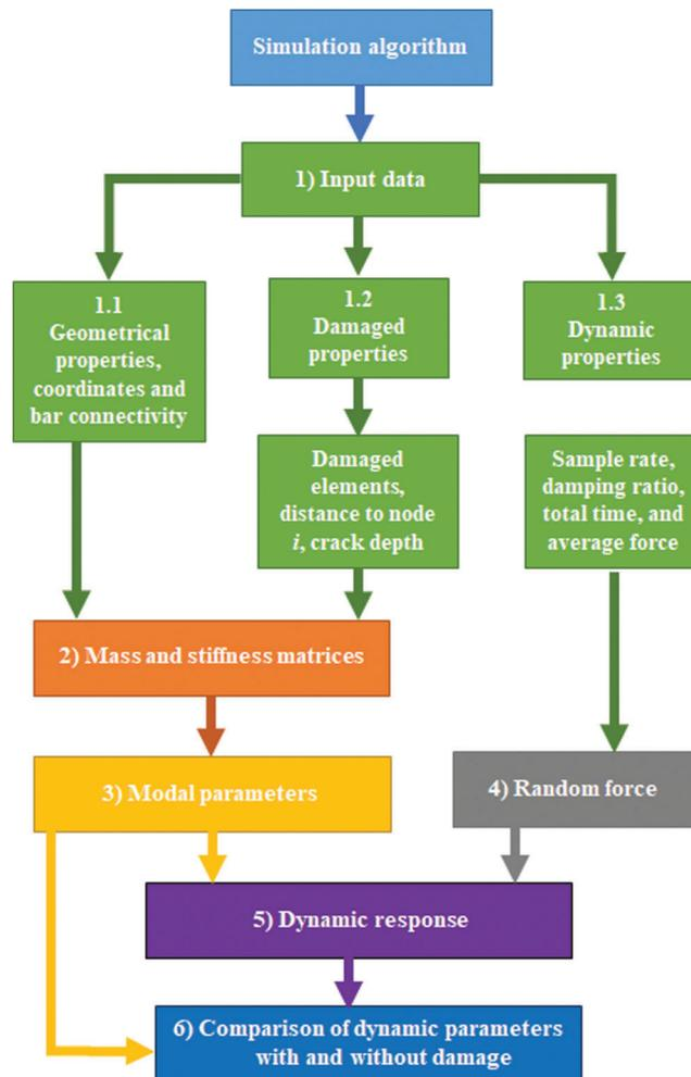
**Figure 2:** Flowchart of the proposed simulation method
