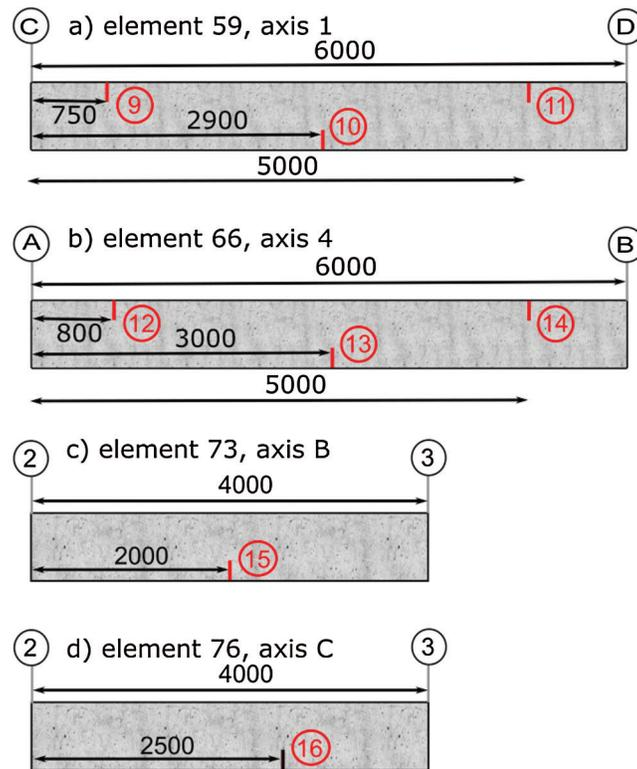
**Figure 8:** Damage location at second level beams (dimensions in mm). a) element 59, axis 1. b) element 66, axis 4. c) element 73, axis B. d) element 76, axis C
