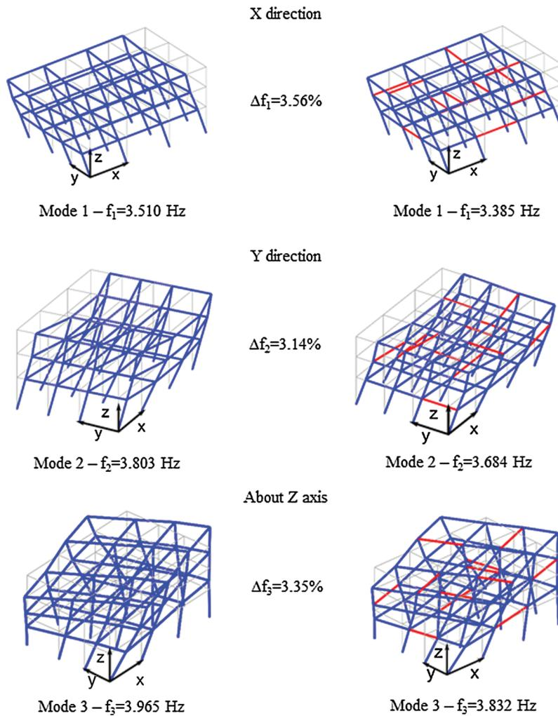
**Figure 11:** Comparison of the first 3 mode shapes of the building without damage (left column) and with damage (elements in red) calculated using the proposed simulation method (right column)
