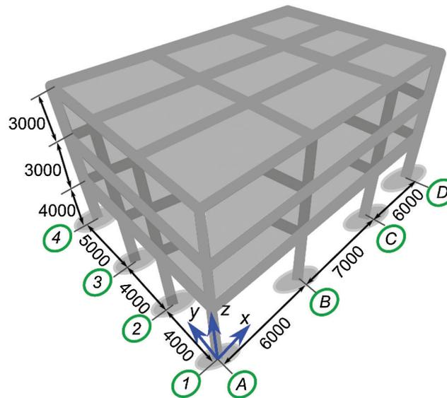
**Figure 5:** Overall geometry of the RC building to be evaluated (dimensions in mm)
