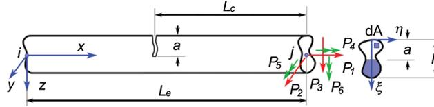
**Figure 1:** Proposed cracked element and forces. Adapted from [4]
