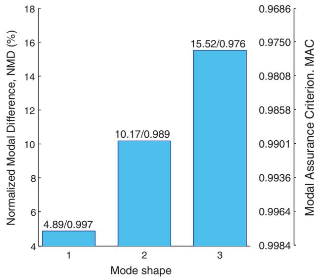
Figure 13: DMN and MAC results for the first 3 mode shapes of the damage scenario
