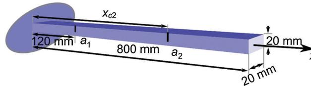
**Figure 3:** Experimental beam adopted for the calibration of the proposed method. Data taken from [17]
