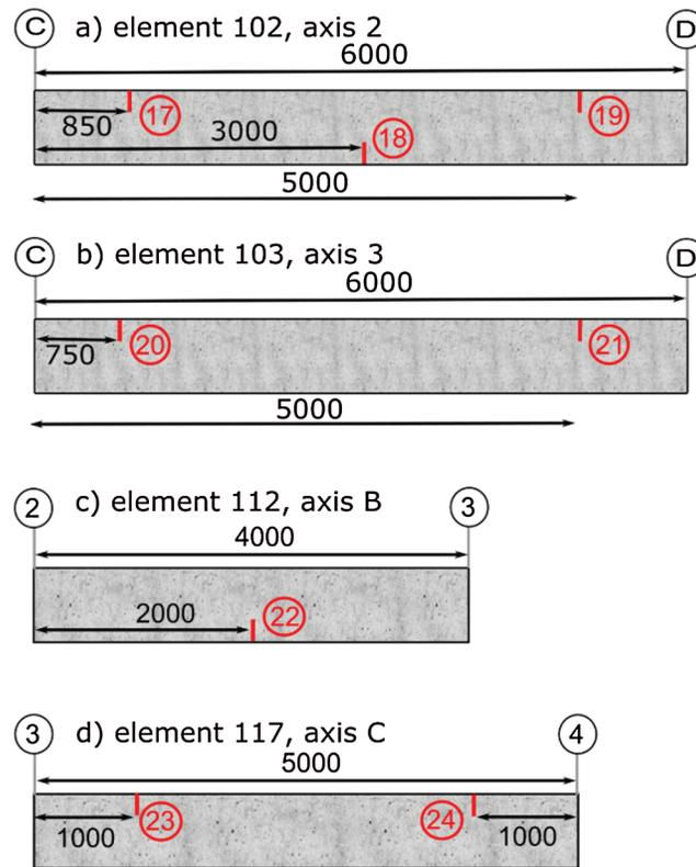
**Figure 9:** Damage location at third level beams (dimensions in mm). a) element 102, axis 2. b) element 103, axis 3. c) element 112, axis B. d) element 117, axis C
