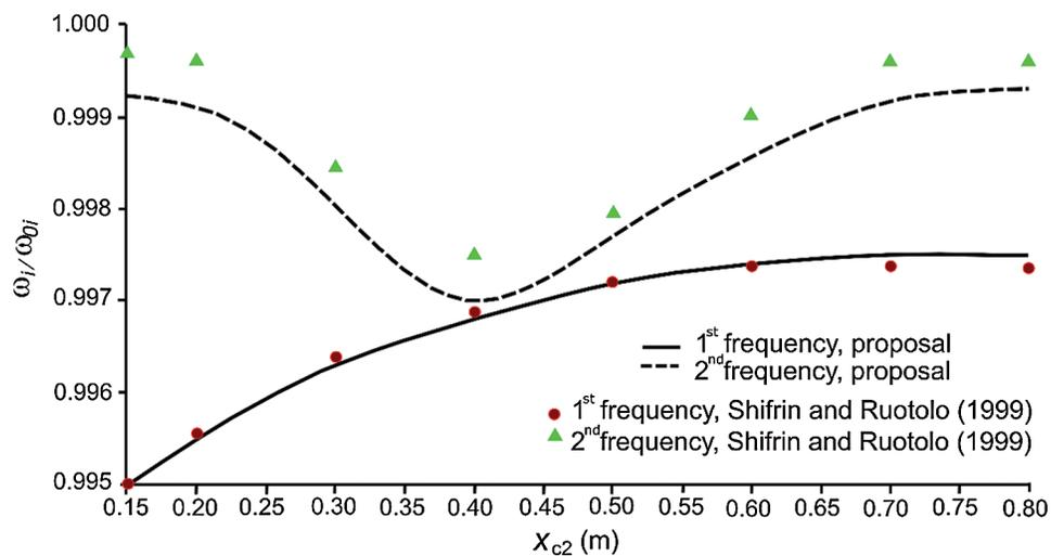
**Figure 4:** Comparison of frequency differences with and without damage of an experimental beam and result from 2 simulation methods. Adapted from [17]
