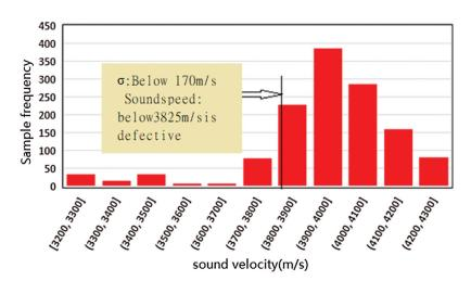
Figure 9: Distribution of sound speed in all columns
