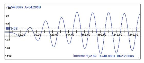
Figure 6: Received waveforms of defect-free concrete
