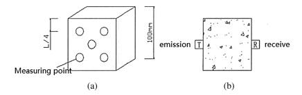
Figure 3: Measuring point layout
