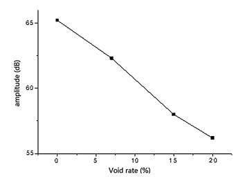
Figure 8: Curves of the variation of the amplitude of the specimens with different emptying rates
