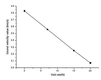
Figure 5: Curves of sound speed values for specimens with different voidage rates
