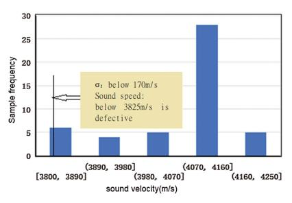
Figure 10: Sound velocity distribution of column part A
