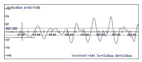
Figure 7: Received waveforms of defective concrete
