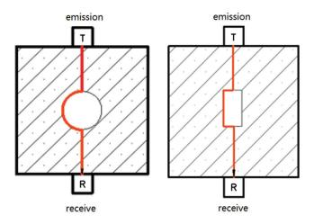
Figure 1: The propagation path of ultrasonic waves in defective concrete. (a) Round defect, (b) Rectangular defect
