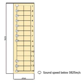
Figure 12: Pillar B test result diagram
