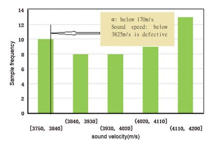
Figure 11: Sound velocity distribution of column part B
