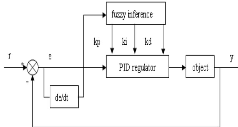
**Figure 5:** Tuning PID parameters of the BP Network
