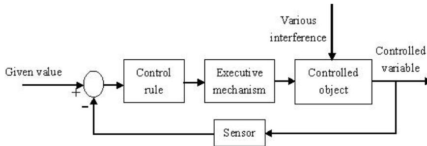
**Figure 1:** Schematic of the heating furnace control system
