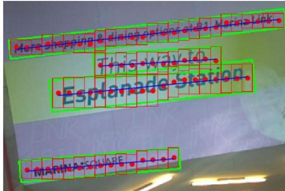
**Figure 5:** The detect results of multi-orientation text with small tilt
